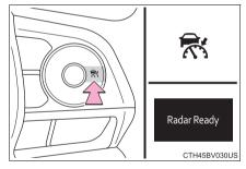
If the cruise control main switch is pressed and held for 1.5 seconds or more, the system turns on in constant speed control mode. (→P. 292)
