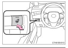
The heated steering wheel can be used when the power switch is in ON mode.
