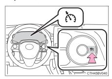
Switching to constant speed control mode is only possible when operating the switch with the cruise control off.
