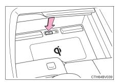
When the power switch is turned off, the on/off state of the wireless charger will be memorized.
