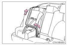
6 If the child restraint has a top tether strap, the top tether strap should be latched onto the top tether strap anchor. (→P. 65)
