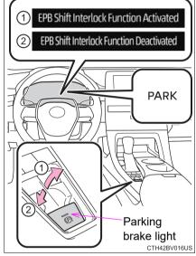
2 Turns automatic mode off (while the vehicle is stopped, press and hold the parking brake switch until a message is shown on the multi-information display)
