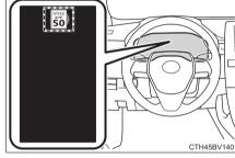
If signs other than speed limit signs are recognized, they will be displayed in an overlapping stack under the current speed limit sign.
