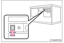
Press and hold the desired HomeLink® button (inside the vehicle) for 2 seconds and release it. Repeat this sequence (press/hold/release) up to 3 times to complete programming.
