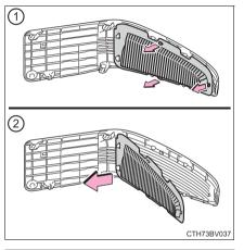
5 Remove the dust and clogs from the filter using a vacuum cleaner, etc.
