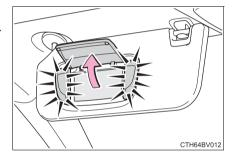
If the vanity lights remain on for 20 minutes while the hybrid system is off, the lights will turn off automatically.
