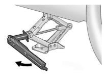
10. Raise the vehicle by turning the jack handle clockwise. Raise the vehicle far enough off the ground so there is enough room for the road tire to clear the ground.
