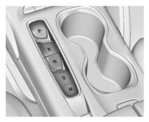
The shift switches are on the center console. The selected gear position will illuminate red on the shift switch, while all others will be displayed in white. If the shift is not immediate, as in very cold conditions, the indicator on the shift switch may flash until it is fully engaged.
