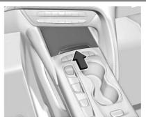
To open the front storage compartment, slide the cover forward. There are two USB ports, SD card slot, and a power outlet inside. To close, push the cover forward and let go.
