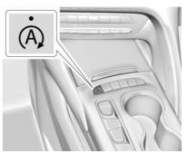
The automatic engine Stop/Start feature can be disabled and enabled by pressing  $\bigwedge$ . Auto Stop/Start is enabled each time you start the vehicle.
