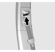
Press and hold the release button while raising or lowering the height adjuster to the desired position. After the height adjuster is set to the desired position, try to move it down without pressing the release button to make sure it has locked into position.
