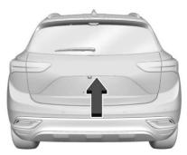
To open the liftgate, press a on the power door lock switch or press a on the remote key twice to unlock all doors. Press the touchpad on the underside of the liftgate handle and lift up.
