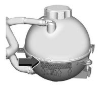
Check to see if coolant is visible in the coolant surge tank. If the coolant inside the coolant surge tank is boiling, do not do anything else until it cools down. If coolant is visible but the coolant level mark is not at or above the indicated mark, add a 50/50 mixture of clean, drinkable water and DEX-COOL coolant. Be sure the cooling system is cool before this is done. See *Engine Overheating*  $\Rightarrow$  262.
