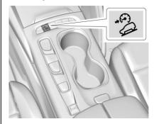
Press  $\stackrel{o}{\Rightarrow}$  to enable or disable HDC. Vehicle speed must be below 50 km/h (31 mph).
