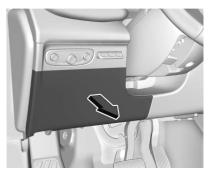
The instrument panel fuse block is on the driver side of the instrument panel, between the steering wheel and the door. To access the fuses, remove the panel, starting at the top. Once clips are disengaged, the tabs along the bottom of the door can be disengaged from the instrument panel to remove the door.
