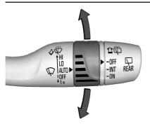
**AUTO :** Move the windshield wiper lever to AUTO. Turn the band on the wiper lever to adjust the sensitivity.
