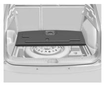
Press the handle, pull up the load floor, and fold forward to access.
