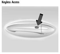
The remote key must be within 1 m (3 ft) of the liftgate or door being opened. Press the button on the door handle to open. See *Remote Key Operation*  $\Rightarrow$  8.
