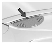
The vehicle has a light sensor on the top of the instrument panel that controls the automatic headlamp system. Do not cover the sensor, otherwise the headlamps may come on when they are not needed.
