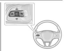
S: Press to turn cruise control on or off. A white indicator comes on in the instrument cluster when cruise control is turned on.
