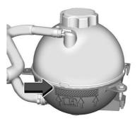
3. If topping off the level in the coolant surge tank, add the proper mixture until the level reaches the mark on the front of the tank and replace the cap. Operate the vehicle. Repeat steps 1–3, as necessary.
