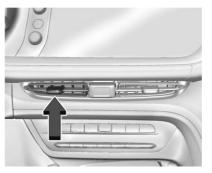
Move the slider knobs to change the direction of the airflow and to shut off the air flow.
