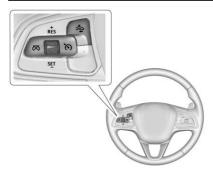
(G) : Press to turn the system on or off. The indicator turns white on the instrument cluster when ACC is turned on.
