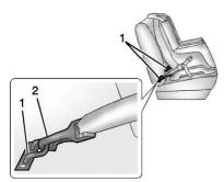
Lower anchors (1) are metal bars built into the vehicle. There are two lower anchors for each LATCH seating position that will accommodate a child restraint with lower attachments (2). **Top Tether Anchor**
