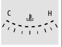
This gauge measures the temperature of the vehicle's engine.
