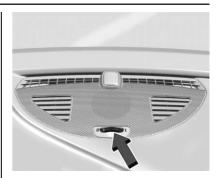
Use the thumbwheel near the air vents to control the amount of airflow or to shut off the airflow.
