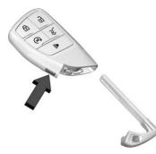
To remove the mechanical key, press the button on the side of the remote key, and pull the mechanical key out. Never pull the mechanical key out without pressing the button.
