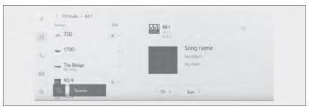
[Ch]: Touch [-] or [+] to search for the receivable broadcasting stations. Touch and hold to jump to the next frequency with available radio signal. When released, the broadcasting station closest to that position with the best reception sensitivity is selected automatically.
