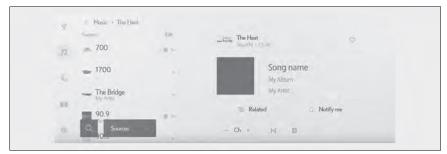
[Ch]: Touch [ — ] or [ + ] to search for the receivable channels. Touch and hold to jump to the next frequency with available radio signal. When released, the current channel is received.
