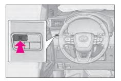
The VIEW switch is located as shown in the illustration.
