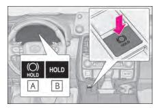
Turns the brake hold system on
