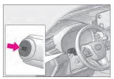
Press the Automatic High Beam switch.
