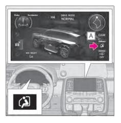
If the engine switch is turned off within approximately 30 seconds after the vehicle is stopped while easy access mode is on, the vehicle height is lowered automatically.
