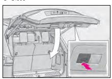
Press the switch on the lower part of the back door.
