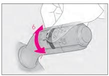
When AUTO is selected, the sensor sensitivity can be adjusted by turning the switch ring.
