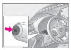
1 Press the Automatic High Beam switch.
