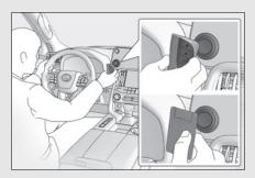
2 Touch the electronic key or card key (if equipped) to the engine switch as shown in the illustration.
