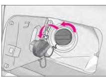
Turn the fuel tank cap slowly to open it and put it into the holder on the fuel filler door.
