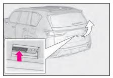
When the back door is unlocked: Press the back door opener switch.
