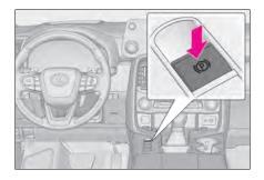
While the vehicle is stopped and depressing the brake pedal, press and hold the parking brake switch until a buzzer sounds and "EPB Shift Interlock Function Deactivated" is displayed on the multi-information display.
