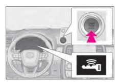
4 Press the engine switch quickly but fully.
