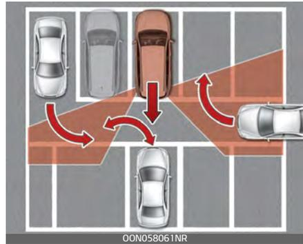
The RCCW/RCCA may not operate properly when the vehicle is in a complex parking environment.
