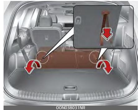
5. To use the rear seat, lift and pull the seatback backward by pulling on the folding lever (for 2nd row) or strap (for 3rd row). Pull the seatback firmly until it clicks into place. Make sure the seatback is locked in place.
