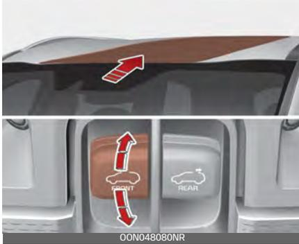
The sunroof will open only while pressing the control switch upward. Move the control switch forward to close the sunroof.
