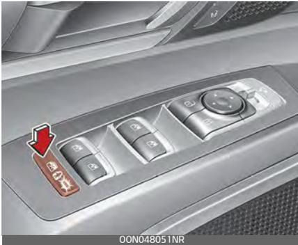
To cancel the electronic child safety lock system, push the electronic child safety lock system switch one more time and then the indicator turns off.
