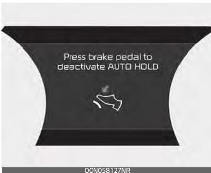
When you press the [AUTO HOLD] switch, if the driver's door and engine hood are not closed or the liftgate is not closed, a warning will sound and a message will appear on the LCD display.
