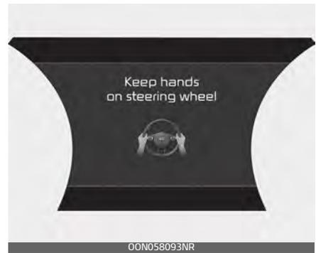
The hands-off warning appears when the system detects that the driver's hands are not on the steering wheel while the HDA is in work. (First warning: warning message, Second warning: warning message with warning sound)
