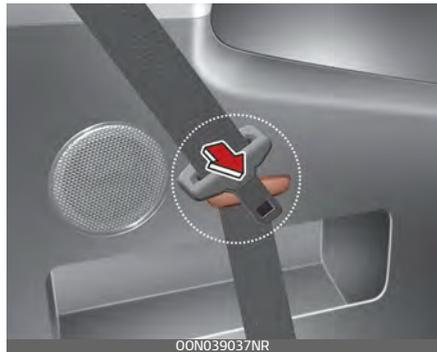
2. After inserting the seat belt, tighten the belt webbing by pulling it up.
