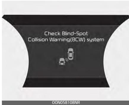
If there is a problem with the BCW, a warning message will appear and the light on the switch will turn off. The RCCW/RCCA will turn off automatically. RCCW and RCCA will not operate also if the BCW turns off due to malfunction. Have your vehicle inspected by an authorized Kia dealer.
