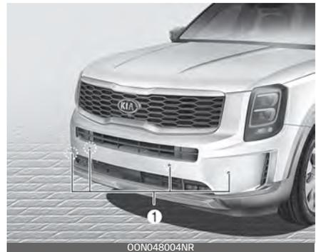
The sensing range and objects detectable by the sensors (1) are limited. Whenever moving while using the parking distance warning, pay as much attention to what is in
