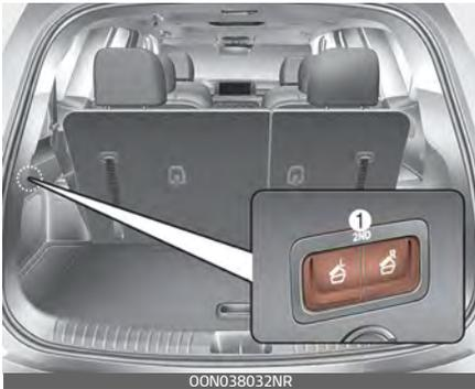
This feature allows you to fold seats in the 2nd row while the liftgate is open.
