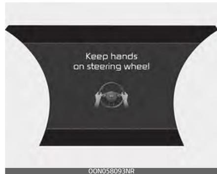
If you keep your hands off the wheel while driving with the LFA is in steering assist mode, the hands-off warning will be triggered.
