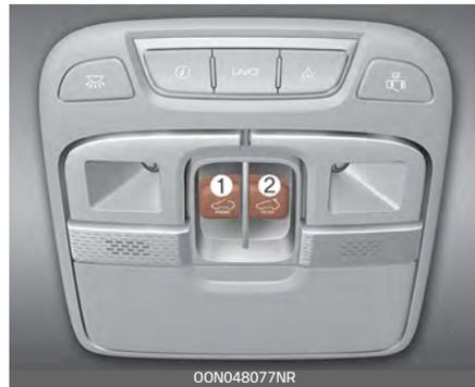
The sunroof can only be opened, closed, or tilted when the ENGINE START/STOP button is in the ON position.
