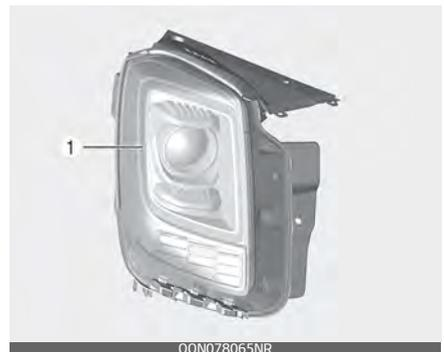
The LED lamps cannot be replaced as a single component because it is an integrated unit. The LED lamps have to be replaced with the unit. A skilled technician should check or repair the position lamp + DRL (LED), for it may damage related parts of the vehicle.
