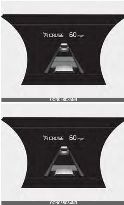
Your vehicle speed will slow down or speed up to maintain the selected distance. (A vehicle will appear in front of your vehicle in the LCD display only when there is an actual vehicle in front of you.)
