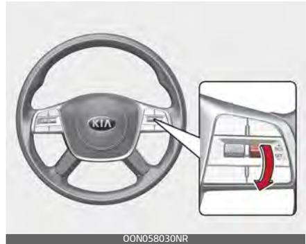
4. Release the accelerator pedal. The desired speed will automatically be maintained.
