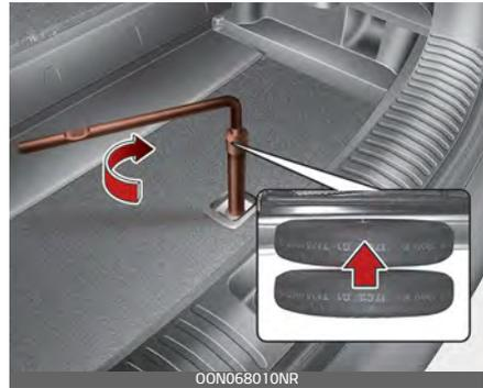
1. Place the wheel under the vehicle and install the retainer through the wheel center.
