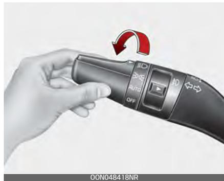
When the light switch is in the headlight position, the head, tail, license lights will turn ON.
