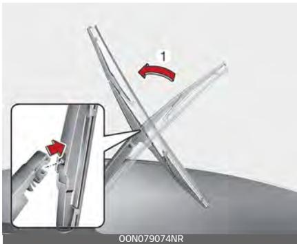
2. Install the new blade assembly by inserting the center part into the slot in the wiper arm until it clicks into place.
