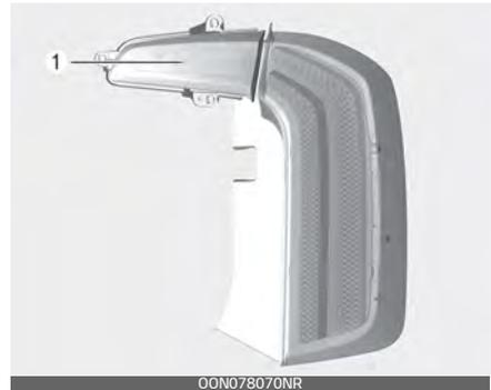
If the Back lamp bulb (Bulb Type) (1) does not operate, have your vehicle checked by an authorized Kia dealer.
