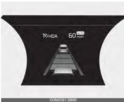
If the HDA operating conditions are all met and setting speed matches with the legal highway speed limit,
