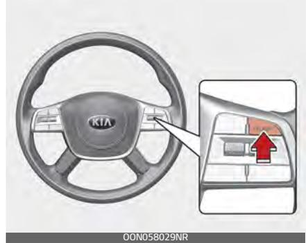
When the SCC is not needed, press the [CRUISE] switch and deactivate the system.
