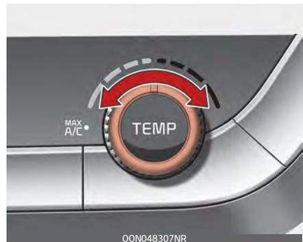
To change the air temperature in the passenger compartment, turn the knob to the right for warm and hot air or to the left for cooler air.
