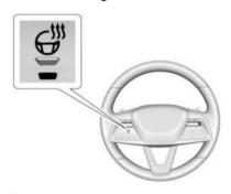
**3**: Press to turn the heated steering wheel on or off. An indicator below the button is lit when the feature is turned on.
