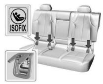
Do not install a child restraint that requires lower anchors in the center rear seating position. See Securing Child Restraints (With the Seat Belt in the Rear Seat) ▷ 76 Securing Child Restraints (With the Seat Belt in the Front Seat) ▷ 78.
