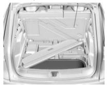
Press the handle and pull up the load floor to access.
