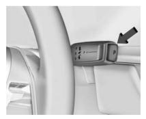
The vehicle uses an electric drive unit. The shift pattern is displayed on the front of the shift lever. The selected gear position will illuminate
