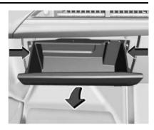
Press the sides of the glove box bin inward to clear the stoppers and turn downward to lower the bin.
