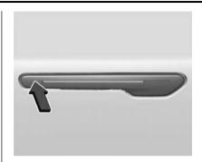
If the door handles are retracted and the remote key is within 1 m (3 ft) of the doors, press a front door handle to deploy the handles.
