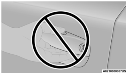
Do NOT Grab The Handle When Locking
