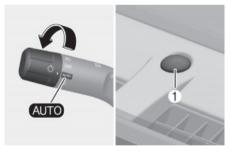
The parking light and headlight are turned ON or OFF automatically depending on the amount of daylight as measured by the ambient light sensor (1) in front of the instrument panel.
