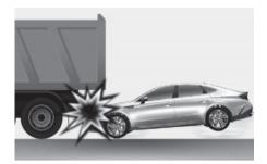
Just before impact, drivers often brake heavily. Such heavy braking lowers the front portion of the vehicle causing it to "nosedive". This is particularly important when the vehicle in front has a higher ground clearance. Airbags may not inflate if your vehicle is in a "nosedive" condition because the collision forces detected by the sensors may have been significantly reduced.
