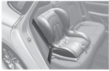
Since all passenger seat belts move freely under normal conditions and only lock under extreme or emergency conditions (emergency locking mode), you must manually pull the seat belt all the way out to shift the retractor to the "Automatic Locking" mode to secure a Child Restraint System.
