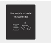
When Highway Driving Assist is operating, your vehicle will stop if the vehicle ahead of you stops. Also, if the vehicle ahead of you starts moving within 30 seconds after the stop, your vehicle will start as well. In addition, after the vehicle has stopped and 30 seconds have passed, the "Use switch or pedal to accelerate" message will appear on the instrument cluster. Depress the accelerator pedal or operate the + switch, - switch or (IIO) switch to start driving.
