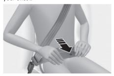
The seat belt automatically adjusts to the proper length after the lap belt portion is adjusted manually so that it fits snugly around your hips. If you lean forward in a slow, easy motion, the belt extends and moves with you.
