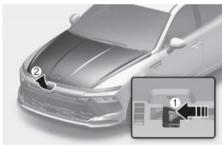
3. Go to the front of the vehicle, raise the hood slightly, push up the secondary hood release lever (1) inside of the hood center and lift the hood (2).
