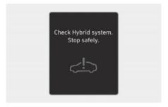
This message appears when there is a problem with the hybrid control system. The **READY** indicator will blink and a warning chime will sound until the problem is solved. Refrain from driving when the warning message appears.
