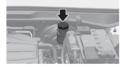
Check the fluid level in the reservoir periodically. The fluid level should be between MAX and MIN marks on the side of the reservoir.
