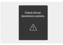
When High Beam Assist is not working properly, the "Check Driver Assistance system" warning message may appear, and the Awarning light may illuminate on the instrument cluster. Have the system inspected by an authorized HYUNDAI dealer.
