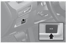
When the trunk is closed, press the power trunk open/close button. The power trunk opens with a warning sound.
