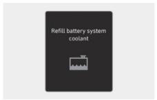
This message appears when the battery system coolant is nearly empty. You should refill the battery system coolant.
