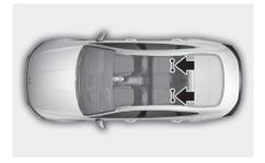
LATCH anchors have been provided in the left and right outboard rear seating positions. Their locations are shown in the illustration. There are no LATCH anchors provided for the center rear seating position.
