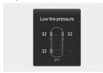
The tire pressure of each tire appears. For more information, refer to the "Tire Pressure Monitoring System (TPMS)" section in chapter 8.
