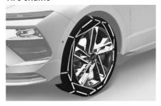
Since the sidewalls of radial tires are thinner than other types of tires, they may be damaged by mounting some types of tire chains on them. Therefore, the use of snow tires is recommended instead of tire chains. If tire chains must be used, install the tire chains after reviewing the instructions provided with the tire chains. Damage to your vehicle caused by improper tire chain use is not covered by your vehicle manufacturer's warranty.
