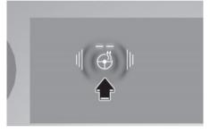
When the Engine Start/Stop button is in the ON position or when the engine is running, press the steering wheel heater button to warm the steering wheel.
