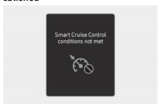
If the Driving Assist button, + switch, - switch or (II'2) switch is operated when Smart Cruise Control operating conditions are not satisfied, the "Smart Cruise Control conditions not met" will appear on the instrument cluster, and an audible warning will sound.
