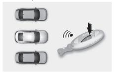
2. Press and hold the Remote Start button ((a)) within 4 seconds until the engine starts.
