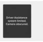
When the front windshield where the front view camera is located is covered with foreign material, such as snow or rain, it can reduce the detecting performance and temporarily limit or disable Intelligent Speed Limit Assist. If this occurs, the "Driver Assistance system limited.
