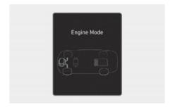
Only the engine power is used to drive the vehicle. (Engine  $\rightarrow$  Wheel)
