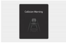
To warn the driver of a collision, the "Collision Warning" warning message appears and the (ﷺ) warning light blinks on the instrument cluster with a warning sound and the steering wheel vibrates.
