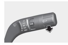
In the OFF position, pull the lever gently toward you to spray washer fluid on the windshield and to run the wipers 1-3 cycles. The spray and wiper operation continues until you release the lever. If the washer does not work, you may need to add washer fluid to the washer fluid reservoir.
