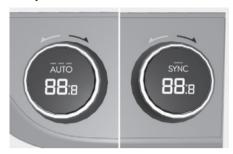
Turn right the knob to increase the temperature. Turn left the knob to decrease the temperature.
