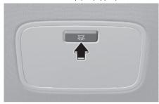
添: Press the button to turn on and off the rear room lamp.
