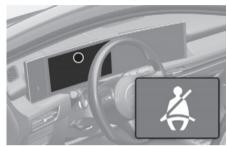
As a reminder to the driver, the driver's seat belt warning light illuminates for about 6 seconds each time the Engine Start/Stop button is in the ON position regardless of seatbelt fastening. If the seatbelt is not fastened, the warning chime will sound for about 6 seconds.
