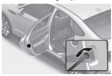
In case of emergency such as when the battery is discharged, the only way to lock the door(s) is with the mechanical key from the outside key hole.
