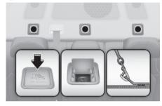
First secure the child restraint with the LATCH lower anchors or the seat belt. If the child restraint manufacturer recommends that the top tether strap be attached, attach and tighten the top tether strap anchor
