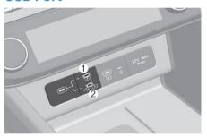
Press the USB port selection button while the engine is running. Press the upper portion of the button (1) to charge an electronic device. Press the lower portion of the button (2) to charge and listen to music with a media storage device. The USB port can be used after either indicator light turns on.
