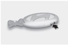
When the trunk is closed, press the power trunk open button for 1 second. The trunk opens with a warning sound.
