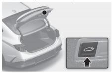
Press the power trunk close button. The trunk will closes automatically.
