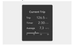
The trip computer mode displays information related to vehicle driving parameters including fuel economy, tripmeter information, and vehicle speed.
