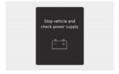
This message appears when a failure occurs in the power supply system. If this occurs, we recommend that your vehicle be inspected by an authorized HYUNDAI dealer.
