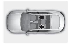
The driver's and front passenger's seats are equipped with adjustable head restraints for the passengers safety and comfort.
