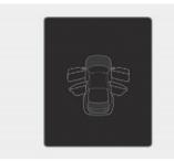
This warning appears if any door or hood or trunk is left open. The warning indicates which door is open on the cluster display.
