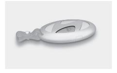
You can start the vehicle using the Remote Start button ((2)) on the smart key.
