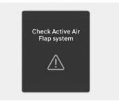
The active air flap system may not operate normally if the air flap is temporarily opened due to foreign factors or if the controller is contaminated by snow or rain, etc.
