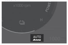
The smart recuperation system is ON and the regenerative braking level appears as "AUTO".
