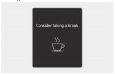
The "Consider taking a break" message will appear and the inattentive driving (") warning light will blink on the instrument cluster with a warning sound to suggest that the driver take a break, when the driver's attention level is below a certain level.
