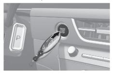
To start the engine, press the Engine Start/Stop button directly with the smart key. If you have a problem with the smart key, contact an authorized HYUNDAI dealer.
