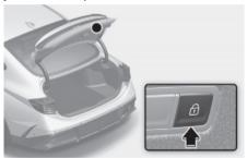
Press the power trunk lock button while carrying the Smart key. The power trunk closes and locks automatically. Additionally, all doors will lock. The trunk will close and lock, and all doors will lock only when the vehicle is off or all doors are closed.
