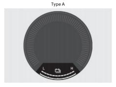
The SOC gauge indicates the remaining hybrid battery power.
