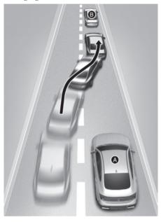
When a vehicle moves into your lane from an adjacent lane, it cannot be detected by the sensor until it is in the sensor's detection range. The smart recuperation system may not immediately detect the vehicle when your vehicle changes lanes abruptly.
