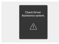
When Safe Exit Warning is not working properly, the "Check Driver Assistance system." warning message will appear on the instrument cluster for several seconds, and the master warning light (A) will appear on the instrument cluster. If this occurs, have your vehicle inspected by an authorized HYUNDAI dealer.
