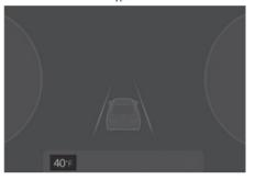
The outside ambient temperature appears in the lower portion of the cluster display. The temperature reads in Fahrenheit or Celsius depending on the units selected from the Settings menu in the instrument cluster or infotainment system.
