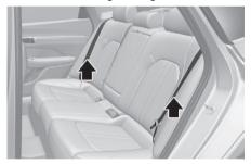
Open the trunk and fold the seat back forward while pulling the seat folding lever (1).
