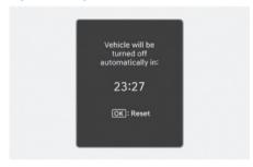
When all the conditions are satisfied, the Vehicle Auto-Shut Off operates and turns the engine off automatically after 60 minutes.
