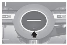
To sound the horn, press the area indicated by the horn symbol on your steering wheel (see illustration). The horn operates only when this area is pressed.
