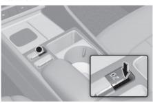
Press and hold the Parking Safety (P<sub>3</sub>) button more than 2 seconds, to turn the Parking Collision-Avoidance Assist on or off.
