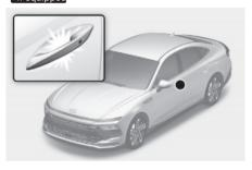
Welcome system helps keep the driver visible by turning on vehicle lights when the driver approaches the vehicle.
