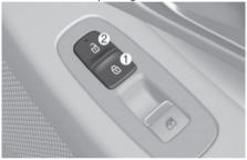
When pressing the  $\Box$  portion (1) on the switch, all vehicle doors are locked.
