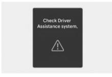
When Lane Following Assist is not working properly, the **Check Driver Assistance system.** warning message will appear on the instrument cluster for several seconds, and the master (△) warning light appears on the instrument cluster. If this occurs, have your vehicle inspected by an authorized HYUNDAI dealer.
