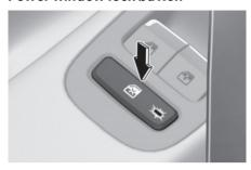
The driver can disable the power window switches on the rear passenger doors by pressing the power window lock button.
