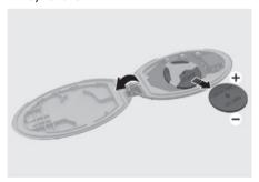
3. Reinstall the rear cover of the smart key.
