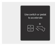
In traffic, your vehicle will stop if the vehicle ahead of you stops. Also, if the vehicle ahead of you starts moving, your vehicle will start as well. In addition, after the vehicle has stopped and a certain time have passed, the "Use switch or pedal to accelerate" message will appear on the instrument cluster. Depress the accelerator pedal or operate the + switch, - switch or (IIO) switch to start driving.
