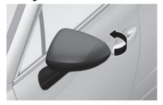
To fold the side view mirror, grasp the housing of the mirror and then fold it toward the rear of the vehicle.
