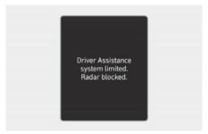
When the rear bumper around the rear-side radar or sensor is covered with foreign material, such as snow or rain, or installing a trailer or carrier, it can reduce the detecting performance and temporarily limit or disable Rear Cross-Traffic Collision-Avoidance Assist.
