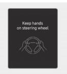
If the driver takes their hands off the steering wheel for several seconds, the "**Keep hands on steering wheel**" warning message appears on the instrument cluster, and an audible warning sounds in stages.
