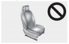
If large quantity of liquid has been spilled on the passenger seat, the airbag warning light may illuminate or malfunction. Therefore, make sure the seat has been completely dried before driving the vehicle.
