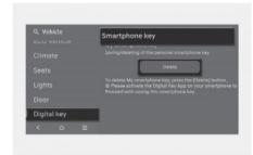
To delete only my registered digital key (smartphone), from the Settings menu select Setup > Vehicle > Digital Keys > Smartphone key > My Smartphone Key > Delete in the infotainment system.
