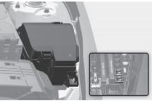
Pull the suspected fuse straight out.
