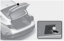
When the trunk is closed, press the power trunk open/close button to open the trunk.
