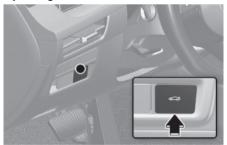
When the trunk is closed, press the trunk open button to open it.
