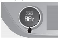
2. Turn left or right the temperature control knob to set the desired temperature. If the temperature is set to the lowest setting, the air conditioning system operates continuously. After the interior has cooled sufficiently, adjust the knob to a higher temperature set point whenever possible.
