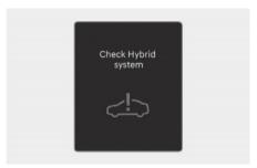
This message appears when there is a problem with the hybrid control system. Refrain from driving when the warning message appears.
