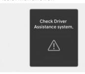
When Blind-Spot Collision-Avoidance Assist is not working properly, the "Check Driver Assistance system." warning message will appear on the instrument cluster for several seconds, and the master (A) warning light will appear on the instrument cluster. If this occurs, have your vehicle inspected by an authorized HYUNDAI dealer.
