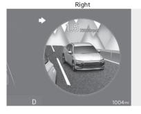
Blind-Spot View Monitor uses the wide-side view cameras to display the rear blind spot areas of your vehicle on the instrument cluster when the turn signal is turned on to help with safe lane changes.
