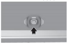
Press the front windshield defroster button (indicator light ON) to turn on the front windshield defroster. If the windshield defogging is set, outside (fresh) mode is automatically selected and the air conditioning turns on according to the detected ambient temperature
