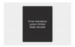
When the front windshield where the front view camera is located, front radar cover, or sensor is covered with foreign material, such as snow or rain, it can reduce the detecting performance and temporarily limit or disable Forward Collision-Avoidance Assist.
