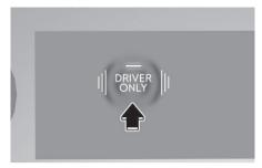
If you press the **DRIVER ONLY** button and the indicator light illuminates, air mostly blows in the direction of the driver's seat.
