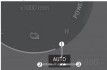
When the smart recuperation system is ON, the regenerative braking level appears as "AUTO" on the instrument cluster. The "AUTO" appears in grey in the ready state. The system automatically controls the regenerative braking level (2) according to the smart recuperation system operating conditions. If the front radar detects a vehicle in front, the indicator light (3) appears in green.
