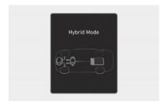
Both the motor and the engine power are used to drive the vehicle. (Battery & Engine → Wheel)
