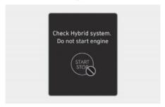
This message appears when the hybrid battery power (SOC) level is low. A warning chime will sound until the problem is solved. Refrain from driving when the warning message appears. If this occurs, we recommend that your vehicle be inspected by an authorized HYUNDAI dealer.
