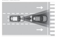
Forward Collision-Avoidance Assist helps detect a vehicle, a powered two-wheeler, a pedestrian, or a cyclist ahead on the road and may warn you of a possible collision with a warning message on the instrument cluster and a warning sound. Also, Forward Collision-Avoidance Assist may assist with braking your vehicle to help reduce collision speed or avoid a collision.
