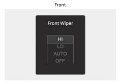
This indicator displays which wiper speed is selected using the wiper control.
