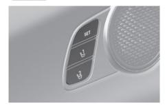
The IMS, or Integrated Memory System, for the driver's seat is provided to store and recall the following memory settings with a simple button operation.
