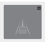
If the vehicle ahead and/or both lane markings are detected and your vehicle speed is below 120 mph (200 km/h), the green (②) indicator light appears on the instrument cluster, and Lane Following Assist helps center the vehicle in the lane by assisting the steering wheel.
