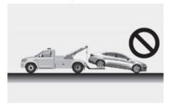
Do not tow vehicles with sling-type equipment. Only use wheel lift or flatbed equipment.
