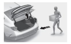
On a vehicle equipped with a smart key, the trunk can be opened with hands-free activation using the smart trunk system.
