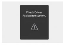
When Lane Keeping Assist is not working properly, the "Check Driver Assistance system." warning message and yellow Lane Keeping Assist (A) warning light appears on the instrument cluster. If this occurs, have your vehicle inspected by an authorized HYUNDAI dealer.
