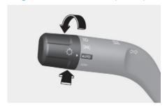
Hight Beam Assist automatically switches between high beam and low beam depending on the detected brightness from the lights of oncoming vehicles or vehicles in front.
