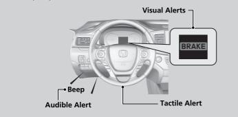
At system's earliest collision alert stage, you can change the distance (**Long/Normal/Short**) between vehicles at which alerts will come on through the audio/information screen setting options.
