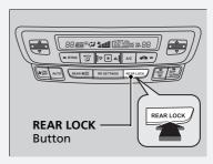
Press the **REAR LOCK** button to turn the rear lock mode on and off.
