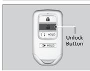
**To open:** Press the unlock button, and then within 10 seconds, press it again and hold it.
