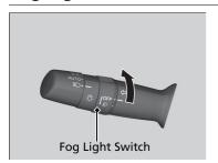
When the headlights are on, turn the fog light switch on to use the fog lights.
