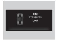
**Tire Pressures Low** is displayed when a tire has significantly low pressure. The specific tire is displayed on the screen.
