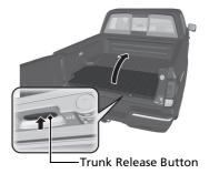
Press the trunk release button to unlock and open the trunk.
