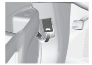
Locate the hood latch lever, pull it up, and then raise the hood. Once you have raised the hood slightly, you can release the lever.
