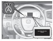
The engine then restarts once the vehicle is about to move again, and the indicator (green) goes off.
