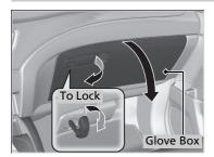
Pull the lever to open the glove box. You can lock the glove box with the built-in key.
