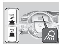
The bed lights can be turned on or off by pressing the button when the transmission is in  $\lceil \mathbf{P} \rceil$ .
