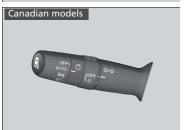
The headlights come on when you unlock a door in dark areas with the headlight switch in **AUTO**.
