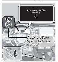
To turn the Auto Idle Stop system off, press this button. The Auto Idle Stop system stops.
