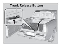
Push up the trunk release button on the trunk lid after all the doors are unlocked.
