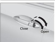
**To open:** Unlock the driver's door with the key. Within 10 seconds of returning the key to the central position, turn the key in the unlock direction and hold it there.
