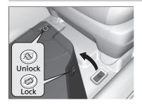
The front and rear seat floor mats hook over the floor anchors, which keep mats them from sliding forward. To remove a mat for cleaning, turn the anchor knobs to the unlock position. When reinstalling the mat after cleaning, turn the knobs to the lock position.
