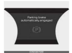
If the driver turns the engine off by mistake while Auto Hold is operating, EPB will be automatically applied. But if the driver turns the engine off and push the EPB switch in 1 second, the EPB does not apply.
