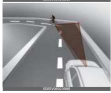
The front view camera or radar sensor recognition function may not detect the vehicle, pedestrian or cyclist travelling in front on a curved road.
