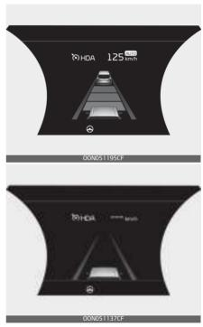
If both lanes are recognized properly (lane color: white), the steering wheel indicator ( ) lights up in green and then the steering control is initiated. When the function can-
