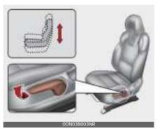
To change the height of the seat cushion, push the lever upwards or
