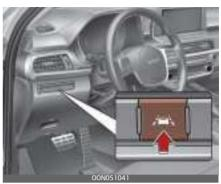
With the ENGINE START/STOP button in the ON position, press the Lane Safety button located on the instrument panel to turn on Lane Keeping Assist. The white indicator light ( ) will illuminate on the cluster. Press the button again to turn off the function.
