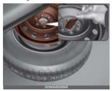
5. Remove the retainer from the center of the spare tire.
