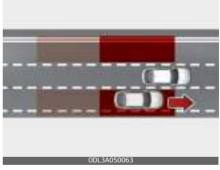
Blind-Spot Collision-Avoidance Assist help detects and informs the driver that a vehicle is in the blind spot.
