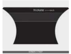
You can see the status of the Smart Cruise Control operation in the Driving Assist view on the cluster. Refer to "Instrument cluster" on page 4-71.
