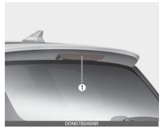
The LED lamps cannot be replaced as a single component because it is an integrated unit. The LED lamps have to be replaced with the unit.
