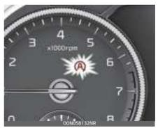
The ISG may not operate when an ISG related sensor or system error occurs.
