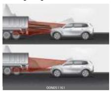
When the vehicle in front has heavy loading extended rearward, or when the vehicle in front has higher ground clearance, it may induce a hazardous situation.
