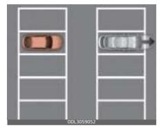
If a vehicle parked in front drives away from you, Leading vehicle departure alert may warn you that the parked vehicle is driving away. When driving at a tollgate or intersection, etc.
