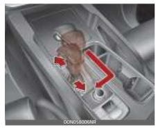
In Manual mode, moving the shift lever backwards or forwards will allow you to make gearshifts rapidly. In contrast to a manual transmission, the Manual mode allows gearshifts with the accelerator pedal depressed.
