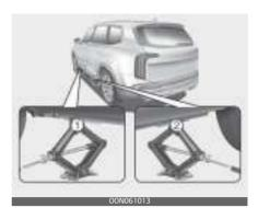
8. Insert the wheel lug nut wrench into the jack and turn it clockwise, raising the vehicle until the tire just clears the ground. This measurement is approximately 30 mm (1 in).
