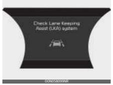
When Lane Keeping Assist is not working properly, the 'Check Lane Keeping Assist (LKA) system', warning message will appear and the yellow ( ) indicator light will illuminate on the cluster. In this case, have the function checked by an authorized Kia dealer.
