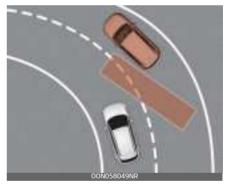
Blind-Spot Collision-Avoidance Assist may not operate properly when driving on a curved road. The function may not detect the vehicle in the next lane.
