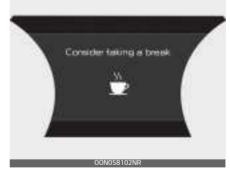
The 'Consider taking a break' message will appear on the cluster and an audible warning will sound to suggest that the driver take a break, when the driver's attention level is below 1.  Driver Attention Warning will not suggest a break when the total driving time is shorter than 10 minutes or 10 minutes has not passed after the last break was suggested.
