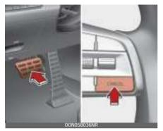
Press the CANCEL button or depress the brake pedal to temporarily cancel Smart Cruise Control
