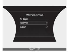
With the ENGINE START/STOP button in the ON position, press MODE button (□) several times on the steering wheel until 'User Settings' menu appears on the LCD display. Select 'Driver Assistance → Warning Timing' to change the initial warning activation time for Blind-Spot Collision-Avoidance Assist
