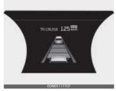
If temporary deceleration is required in the standby state and Navigation-based Smart Cruise Control is operating, the green (AUTO) symbol will illuminate on the cluster.
