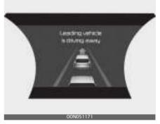
While Smart Cruise Control is in operation if your vehicle stops behind the vehicle in front, the vehicle in front depart from a stop, Leading vehicle departure alert will inform the driver by displaying the 'Leading vehicle is driving away' message on the cluster and an audible warning will sound.
