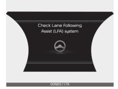
When Lane Following Assist is not working properly, the 'Check Lane Following Assist (LFA) system' warning message will appear on the cluster (turns off after a certain time) and ( ) warning light will illuminate.
