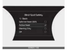
With the ENGINE START/STOP button in the ON position, press MODE button (□) several times on the steering wheel until 'User Settings' menu appears on the LCD display. Select 'Driver Assistance → Blind-Spot Safety' from the setting menu to set whether or not to use each function
