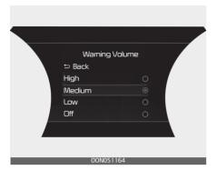
With the ENGINE START/STOP button in the ON position, press MODE button (□) several times on the steering wheel until 'User Settings' menu appears on the LCD display. Select 'Driver Assistance → Warning Volume' to change the warning volume to 'High', 'Medium', 'Low' or 'Off' for Lane Keeping Assist.
