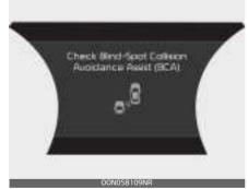
When Blind-Spot Collision-Avoidance Assist is not working properly, the 'Check Blind-Spot Collision Avoidance Assist (BCA)' warning message will appear (turns off after a certain time), and (\(\begin{aligned} \begin{aligned} \text{\text{off}} \end{aligned} \) warning light will illuminate on the cluster. In this case, have your vehicle inspected by an authorized Kia dealer.
