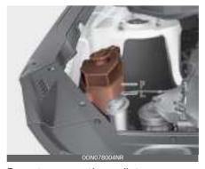
Do not remove the radiator cap when the engine and radiator are hot. Scalding hot coolant and steam Maintenance Engine coolant
