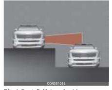
Blind-Spot Collision-Avoidance Assist may not operate properly when driving where the heights of
