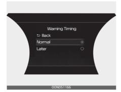
With the ENGINE START/STOP button in the ON position, press MODE button (□) several times on the steering wheel until 'User Settings' menu appears on the LCD display. Select 'Driver Assistance → Warning Timing' to change the initial warning
