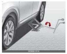
Before removing the wheel lug nuts, make sure the vehicle is s and that there is no chance for movement or slippage.
