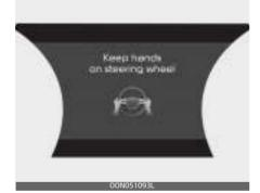
If the driver takes their hands off the steering wheel for several seconds, the 'Keep hands on steering wheel' warning message will appear on the cluster, and an audible warning will sound in stages.
