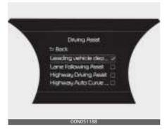
If 'Leading vehicle departure alert' is selected from 'Driver Assistance → Driving Assist', the function will inform the driver when the front vehicle departs from a stop.
