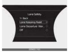
With the ENGINE START/STOP button in the ON position, press MODE button (□) several times on the steering wheel until 'User Settings' menu appears on the LCD display. Select 'Driver Assistance → Lane Safety' from the setting menu to set whether or not to use each function.
