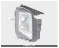
The LED lamps cannot be replaced as a single component because it is an integrated unit. The LED lamps have to be replaced with the unit. A skilled technician should check or repair the position lamp + DRL (LED), for it may damage related parts of the vehicle.
