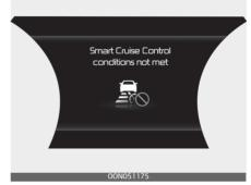
If the Driving Assist button, RES+, SET- switch is pushed when Smart Cruise Control operating conditions are not satisfied, the 'Smart Cruise Control conditions not met' will appear on the cluster, and an audible warning will sound.
