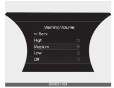
With the ENGINE START/STOP button in the ON position, press MODE button (□) several times on the steering wheel until 'User Settings' menu appears on the LCD display. Select 'Driver Assistance → Warning Volume' to change the warning volume to 'High', 'Medium', 'Low' or 'Off' for Smart Cruise Control.
