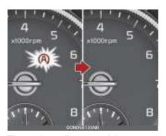
The engine will start and the green AUTO STOP indicator  $(\mathbf{A})$  on the instrument cluster will go out.
