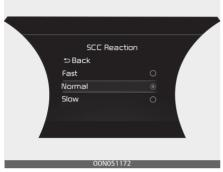
The sensitivity of vehicle speed when following the front vehicle to maintain the set distance can be adjusted. Go to the "User Settings → Driver Assistance → SCC Reaction → Fast/Normal/Slow". You may select one of the three stages you prefer.
