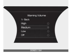
With the ENGINE START/STOP button in the ON position, press MODE button (□) several times on the steering wheel until 'User Settings' menu appears on the LCD display. Select 'Driver Assistance → Warning Volume' to change the warning volume to 'High', 'Medium', 'Low' or 'Off' for Blind-Spot Collision-Avoidance Assist.
