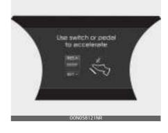
In traffic, your vehicle will stop if the vehicle ahead of you stops. Also, if the vehicle ahead of you starts moving, your vehicle will start as well. In addition, after the vehicle has stopped and a certain time have passed, the 'Use switch or pedal to accelerate' message will appear on the cluster. Depress the accelerator pedal or push the RES+ switch up or push the SET- switch down to start driving.
