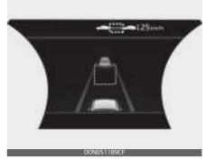
If you want to speed up temporarily when Smart Cruise Control is on, depress the accelerator pedal for a certain amount. While depressing the accelerator pedal for a certain amount, the set speed will blink on the cluster. However, if the accelerator pedal is insufficiently depressed, the vehicle may slow down.
