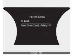
With the ENGINE START/STOP button in the ON position, press MODE button (□) several times on the steering wheel until 'User Settings' menu appears on the LCD display. Select 'Driver Assistance → Parking Safety → Rear Cross-Traffic Safety' from the setting menu to set whether or not to use each function.
