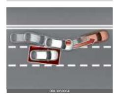
When changing lanes by detecting the lane ahead, if Blind-Spot Collision-Avoidance Assist judges that there is a collision risk with an approaching vehicle in the blind spot, it will help avoid collision by applying the differential brake.
