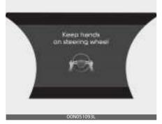
The hands-off warning appears when the function detects that the driver's hands are not on the steering wheel while Highway Driving Assist is in operation.
