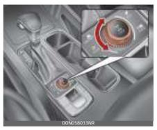
\* When the DRIVE mode is activated by pressing the DRIVE/TERRAIN button, turn the knob to display as shown below.
