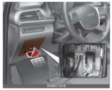
Pull the suspected fuse straight out. Use the removal tool provided on the engine fuse panel cover.
