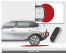
The Smart Power Liftgate operates with a welcome alert if the smart key is detected within 50~100 cm (20~39 inches) from the liftgate.  The alert stops once the smart key is positioned outside the detecting area during the Detect and Alert stage.
