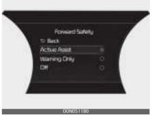
With the ENGINE START/STOP button in the ON position, press MODE button (□) several times on the steering wheel until 'User Settings' menu appears on the LCD display. Select 'Driver Assistance → Forward Safety' from the setting menu to set whether or not to use each function.
