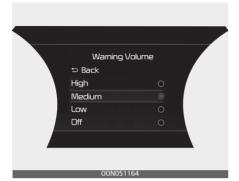
With the ENGINE START/STOP button in the ON position, press MODE button ( several times on the steering wheel until 'User Settings' menu appears on the LCD displau. Select 'Driver Assistance → Warning Volume' to change the warning volume to 'High', 'Medium', 'Low' or 'Off' for Forward Collision-Avoidance Assist.
