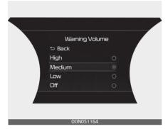
With the ENGINE START/STOP button in the ON position, press MODE button (□) several times on the steering wheel until 'User Settings' menu appears on the LCD display. Select 'Driver Assistance → Warning Volume' to change the warning volume to 'High', 'Medium', 'Low' or 'Off' for Rear Cross-Traffic Collision-Avoidance Assist.
