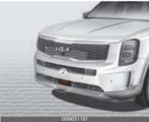
[1]: Front view camera, [2]: Front radar The front view camera and front radar are used as a detecting sensor to detect front vehicles.
