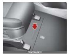
The number is punched on the floor under the passenger seat. To check the number, open the cover.
