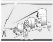
AM and FM radio signals are broadcast from transmitter towers located around your city. They are intercepted by the radio antenna on your vehicle. This signal is then processed by the radio and sent to your vehicle speakers. In some cases the signal coming to your vehicle may not be strong and clear
