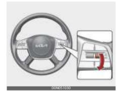
4. Release the accelerator pedal. The desired speed will automatically be maintained. If there is a vehicle in front of you, the speed may decrease to maintain the distance to the vehicle ahead. On a steep grade, the vehicle may slow down or speed up slightly while going uphill or downhill.
