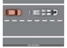
If the vehicle in front abruptly departures, Leading vehicle departure alert may not operate properly.
