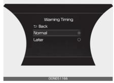
With the ENGINE START/STOP button in the ON position, press MODE button (□) several times on the steering wheel until 'User Settings' menu appears on the LCD display. Select 'Driver Assistance → Warning Timing' to change the initial warning activation time for Rear Cross-Traffic Collision-Avoidance Assist.
