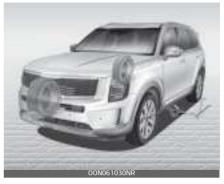
5. Block both the front and rear of the wheel that is diagonally opposite from the jack position.
