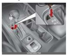
If the shift lever cannot be moved from the P (Park) position into R (Reverse) position with the brake pedal engaged, continue engaging the brake, then do the following:
