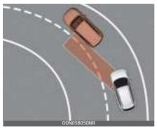
Blind-Spot Collision-Avoidance Assist may not operate properly when driving on the curved road. The function may recognize the vehicle in the same lane.
