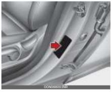
The tire label located on the driver's side center pillar gives the tire pressures recommended for your vehicle.
