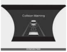
To warn the driver of a collision, the 'Collision Warning' warning message will appear on the cluster, an audible warning will sound
