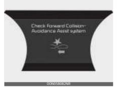
When Forward Collision-Avoidance Assist is not working properly, the 'Check Forward Collision-Avoidance Assist system' warning message will appear (turns off after a certain time), and the and warning lights will illuminate on the cluster. In this case, have the vehicle inspected by an authorized Kia dealer.
