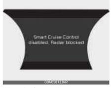
When the front radar cover or sensor is covered with snow, rain, or foreign matters, it can reduce the detecting performance and tempo-
