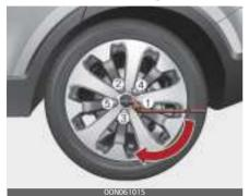
18.After changing wheels, have an authorized Kia dealer tighten the wheel nuts to their proper torque as soon as possible.
