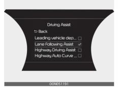
With the ENGINE START/STOP button in the ON position, press MODE button (□) several times on the steering wheel until 'User Settings' menu appears on the LCD display. Select 'Driver Assistance → Driving Assist → Lane Following Assist' from the setting menu to set whether or not to use each function.
