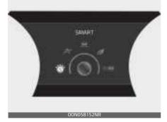
SMART mode: SMART mode automatically adjusts the driving mode (ECO
