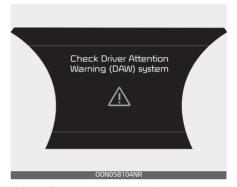
When Driver Attention Warning is not working properly, the 'Check Driver Attention Warning (DAW) system' warning message will appear on the cluster (turns off after a certain time) and (\(\bigcap\)) warning light will illuminate. In this case, have your vehicle inspected by an authorized Kia dealer.
