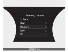
With the ENGINE START/STOP button in the ON position, press MODE button (□) several times on the steering wheel until 'User Settings' menu appears on the LCD display. Select 'Driver Assistance → Warning Volume' to change the warning volume to 'High', 'Medium', 'Low' or 'Off' for Lane Following Assist.
