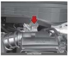
Before removing the reservoir cap and adding brake fluid, clean the area around the reservoir cap thoroughly to prevent brake fluid contamination.
