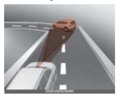
Your vehicle speed can be reduced due to a vehicle in the adjacent lane.
