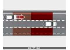
Blind-Spot Collision-Avoidance Assist helps detect and inform the driver that a vehicle is approaching at high speed from the blind spot area.
