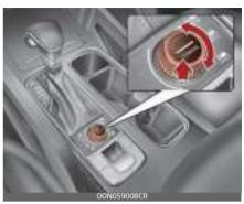
You can switch from DRIVE MODE to TERRAIN mode by pressing DRIVE/TERRAIN mode button and then select SNOW, MUD, or SAND mode by turning TERRAIN MODE knob. If you press the DRIVE/TERRAIN mode button again, the vehicle will go back to DRIVE MODE.
