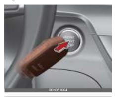
But for your safety always press the brake pedal before starting the engine.
