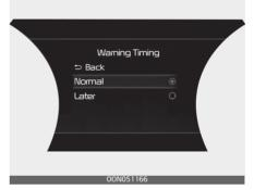
With the ENGINE START/STOP button in the ON position, press MODE button (□) several times on the steering wheel until 'User Settings' menu appears on the LCD display. Select 'Driver Assistance → Warning Timing' to change the initial warning activation time for Forward Collision–Avoidance Assist.
