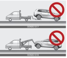
Do not tow the vehicle backwards with the front wheels on the ground as this may cause damage to the transmission. Do not tow with sling-type equipment. Use wheel lift or flatbed equipment.
