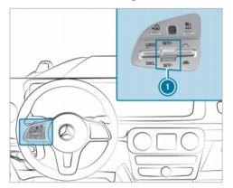
To operate Active Distance Assist DISTRONIC: push the rocker switches on the steering wheel control unit up or down to the desired position.
