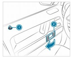
To unlock and open a front door: pull door handle 2. Locking pin 1 pops up when the door is unlocked.
