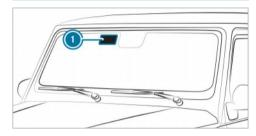
Vehicles with windshield heater: Radio-controlled equipment, such as toll systems, can be mounted only on area (1) of the windshield which is permeable to radio waves.
