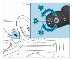
Turn the lever in the direction of arrow or If indicator lamp (3) lights up, the steering
