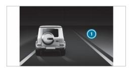
If a lane-correcting brake application occurs, display 1 will appear on the instrument display.
