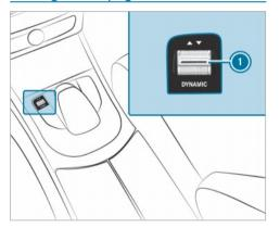
Push DYNAMIC SELECT switch (1) forwards or backwards. The selected drive program appears in the Instrument Display and media display.
