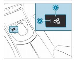
To activate/deactivate: press button ①. If indicator lamp ② is lit, manual gearshifting is activated. Transmission position M and the current gear will appear on the Instrument Display.
