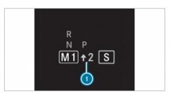
If gearshift recommendation (1) appears next to the transmission position display, shift to the recommended gear.
