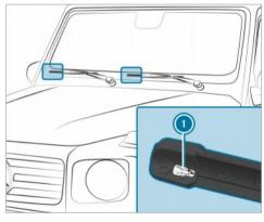
Remove protective film (1) from the maintenance displays on the tips of the newly installed wiper blades.
