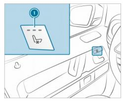
Press button (1) repeatedly until the desired blower setting has been reached. Depending on the blower setting, up to three indicator lamps will light up. If all indicator
