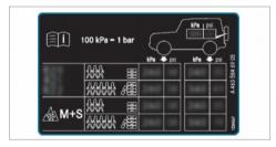
The tire pressure table shows the recommended tire pressure for all tires approved for this vehicle. The recommended tire pressures apply for cold
