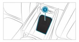
To connect a mobile phone: hold the NFC area of the mobile phone (see manufacturer's operating instructions) on mat o or place the mobile phone on it.
