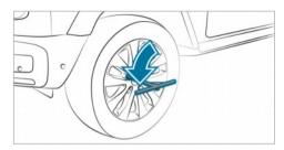
Using the wheel bolt, loosen the wheel bolts on the wheel you wish to change by about one full turn. Do not unscrew the screws completely.
