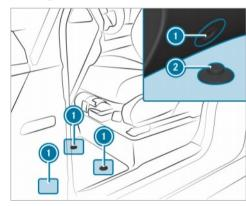
Move the corresponding seat backwards and lay the floor mat in the footwell.
