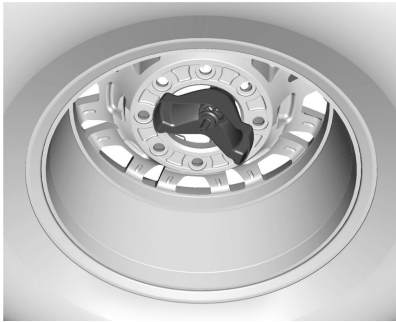
AT4X Model Incorrectly Stored, Retainer Off-Center
