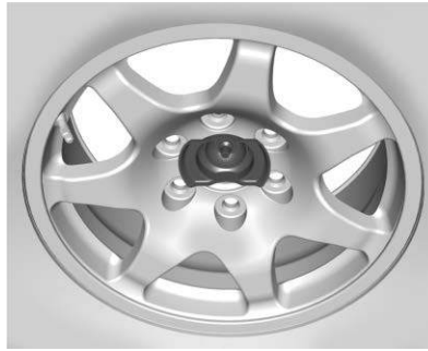
All Other Models Correctly Stored, Retainer Centered
