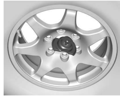
All Other Models Incorrectly Stored, Retainer Off-Center
