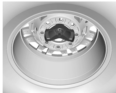
AT4X Model Correctly Stored, Retainer Centered
