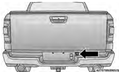
Access Hole Cover Location
