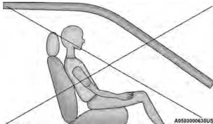
Not Seated Properly
