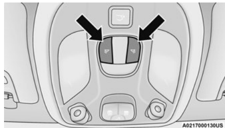
Overhead Light Switches
