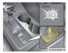
Depress the brake pedal, start the engine and then press the Auto Hold button. The white AUTO HOLD indicator will come on indicating the system is in standby.
