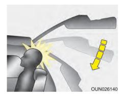
WARNING - 3rd row seat 3rd row occupants should always remain in the center of the seat cushion so the occupants head is protected by the headrest.
