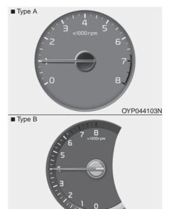
The tachometer indicates the approximate number of engine revolutions per minute (rpm).
