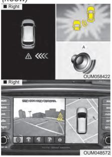
If the vehicle detected by the sensors approaches from the rear left/right side of your vehicle, the warning chime will sound, the warning light on the outside rearview mirror will blink and a message will appear on the LCD display. If the rear view monitor system is in activation, a message will also appear on the 'Car Infotainment System'.
