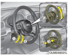
To change the steering wheel angle, pull down the lock-release lever (1), adjust the steering wheel to the desired angle (2) and height (3) then pull up the lock-release lever to lock (4) the steering wheel in place. Be sure to adjust the steering wheel to the desired position before driving.
