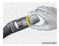
The rear window wiper and washer switch is located at the end of the wiper and washer switch lever. Turn the switch to the desired position to operate the rear wiper and washer.
