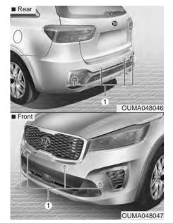
The Parking Distance Warning assists the driver during movement of the vehicle by chiming if any object is sensed within the distance of 39 in. (100 cm) in front and 47 in. (120 cm) behind the vehicle.
