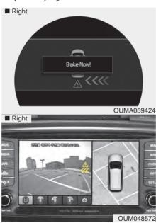
If the risk of collision is detected while the RCCW is generated, brake is controlled. The instrument cluster will inform the driver of the brake control. If the rear view monitor system is in activation, a message will also appear on the 'Car Infotainment System'.
