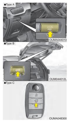
Press the power liftgate close button for approximately one second when the liftgate is opened.
