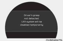
If the driver takes hands off the steering wheel for several seconds while the LKA is activated, the system will warn the driver.
