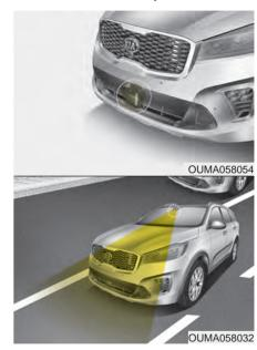
In order for the FCA system to operate properly, always make sure the sensor or sensor cover is clean and free of dirt, snow, and debris.
