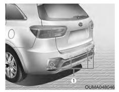
The Reverse Parking Distance Warning assists the driver during backward movement of the vehicle by chiming if any object is sensed within a distance of 47 in. (120 cm) behind the vehicle.
