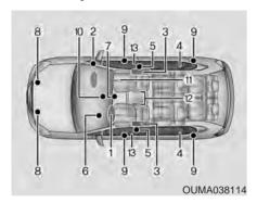
The SRS consists of the following components:
