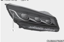
If the side marker (LED) (1) does not operate, have the vehicle checked by an authorized Kia dealer.
