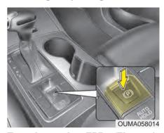
To release the EPB (Electronic Parking Brake), press the EPB switch in the following condition:
