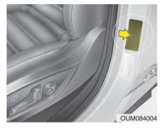
vehicle certification label attached on the driver's side center pillar gives the vehicle identification number (VIN).
