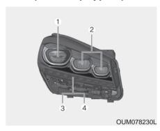
If the Low/High beam lamp(1,2), Front turn signal lamp(3), Day time running lamp/Position lamp(4) does not operate, have the vehicle checked by an authorized Kia dealer.
