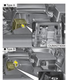
If the main fuse is blown, it must be removed as follows:
