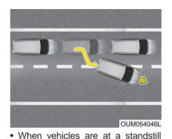
and the vehicle in front of you changes to the next lane, be careful when your vehicle starts to move because it may not recognize the stopped vehicle in front of you. In this case, you must maintain a safe braking distance, and if necessary, depress the brake pedal to reduce your driving speed in order to maintain a safe distance.
