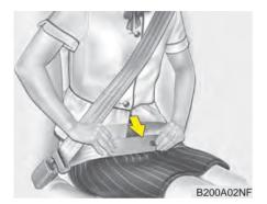
The seat belt automatically adjusts to the proper length only after the lap belt portion is adjusted manually so that it fits snugly around your hips. If you lean forward in a slow, easy motion, the belt will extend and let you move around. If there is a sudden stop or impact, however, the belt will lock into position. It will also lock if you try to lean forward too guickly.
