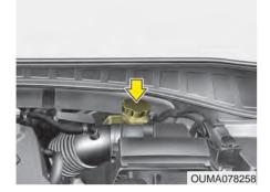
Check the fluid level in the reservoir periodically. The fluid level should be between MAX (Maximum) and MIN (Minimum) marks on the side of the reservoir.
