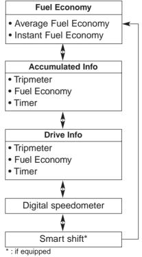
To change the trip mode, scroll the MOVE scroll switch  $(\triangle/\nabla)$  in the trip computer mode.
