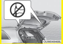
Do not grab the power liftgate struts while the liftgate is open.
