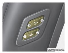
The switch is located on the left side of the front passenger's seatback.
