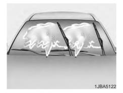
Commercial hot waxes applied by automatic vehicle washes have been known to make the windshield difficult to clean.
