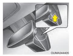
Auto defogging reduces the probability of fogging up the inside of the windshield by automatically sensing the moisture of inside the windshield. The auto defogging system operates
