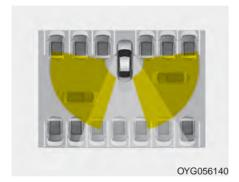
The RCCW uses radar sensors to monitor the approaching cross traffic from the left and right side of the vehicle when your vehicle is in reverse.
