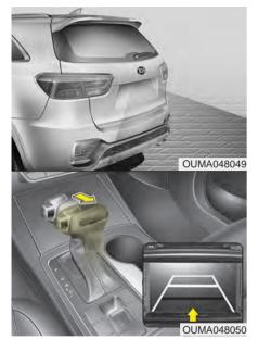
The Rear View Monitor will activate with the ignition switch ON and the shift lever in the R (Reverse) position. This system is a supplemental system that shows behind the vehicle through the rearview display mirror while backing up unless equipped with system that can be displayed rear view, then will display on the screen.
