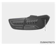
If the side marker (LED) (1) does not operate, have the vehicle checked by an authorized Kia dealer.
