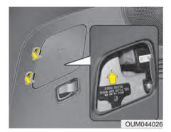
If the fuel filler door does not open using the remote fuel filler door release, you can open it manually. Remove the panel in the cargo area. Pull the handle out slightly.
