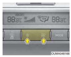
The fan speed can be set to the desired speed by operating the fan speed control button.
