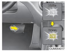
2. When coming to a complete stop by depressing the brake pedal, the AUTO HOLD indicator changes from white to green indicating the AUTO HOLD is engaged and EPB is applied. The vehicle will remain at a standstill even if you release the brake pedal.
