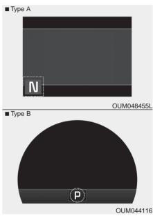
This indicator displays which automatic transmission shift lever is selected.
