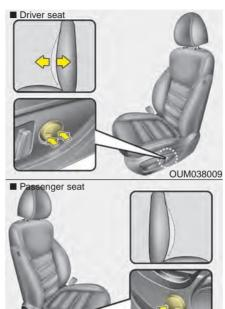
The lumbar support can be adjusted by pressing the lumbar support switch on the side of the seat.
