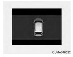
The warning message will appear on the LCD display when hood is open.
