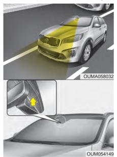
The Lane Keeping Assist System detects the lane markers on the road with a front view camera at the front windshield, and assists the driver's steering to help keep the vehicle in the lanes.
