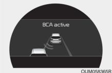
The Blind-Spot Collision-Avoidance Assist (BCA) system may apply braking power, when an approaching vehicle is detected within a certain distance next to/behind your vehicle.
