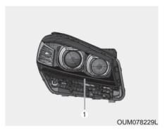
If the position lamp (LED) (1) does not operate, have the vehicle checked by an authorized Kia dealer.
