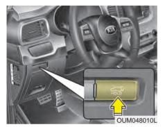
Press the power liftgate open/close button for approximately one second.
