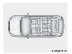
Some child seat manufacturers make child restraint seats that are labeled as LATCH or LATCH-compatible child restraint seats. LATCH stands for "Lower Anchors and Tethers for Children". These seats include two rigid or webbing mounted attachments that connect to two LATCH anchors at specific seating positions in your vehicle. This type of child restraint seat eliminates the need to use seat belts to attach the child seat in the rear seats.
