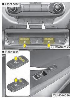
The seat warmer is provided to warm the front seats during cold weather. With the ignition switch in the ON position, push either of the switches to warm the driver's seat or the front passenger's seat. During mild weather or under conditions where the operation of the seat warmer is not needed, keep the switches in the "OFF" position.
