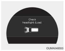
This warning message illuminates if there is a malfunction (burned-out bulb except LED lamp or circuit malfunction) with the headlamp. In this case, have your vehicle inspected by an authorized Kia dealer.
