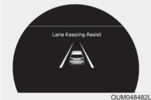
If the speed of the vehicle is over 40 mph (64 km/h) and the system detects lane markers, the color changes from gray to white. When the conditions below are met, LKA system will be enable to assist steering.
