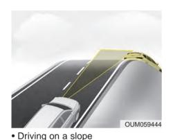
The performance of Forward Collision-Avoidance Assist system may be decreased while driving upward or downward on a slope. The radar sensor recognition may not detect the vehicle in front.
