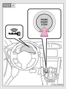
Press the "ENGINE START STOP" switch shortly and firmly.
