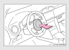
To sound the horn, press on or close to the key mark.
