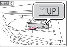
Remove the air conditioning filter and replace it with a new one.
