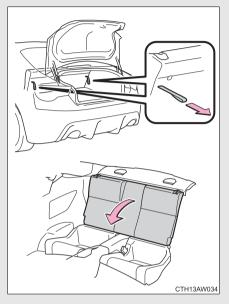
Pull the seatback lock release straps in the trunk for the seatback you wish to fold down.
