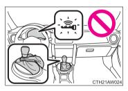
Vehicles with an automatic transmission: Check that the shift lever is securely set in P. The engine may not start if the shift lever is displaced out of P. The smart key system indicator light (green) will flash quickly.
