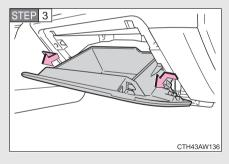
Push in each side of the glove box and pull the glove box toward you to disconnect the claws.
