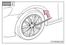
Slightly loosen the wheel nuts (one turn).
