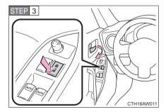
Open the driver's door while pressing and holding on the door lock switch and continue to press for approximately 10 seconds after the driver's door has opened.
