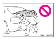
The trunk lid may suddenly shut if it is not opened fully. It is more difficult to open or close the trunk lid on an incline than on a level surface, so beware of the trunk lid unexpectedly opening or closing by itself. Make sure that the trunk lid is fully open and secure before using the trunk.
