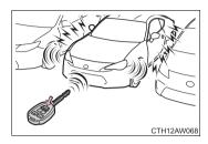
When the function is set, a buzzer (sounds once) and the emergency flashers (flash 3 times) are used to inform the driver of the vehicle's location.
