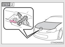
Push the auxiliary catch lever to the left and lift the hood.
