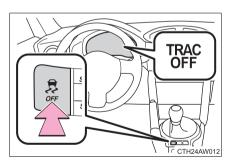
To turn the TRAC system off, quickly press and release the button.
