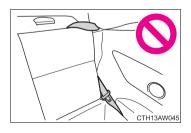
Always make sure that the seat belt is not caught in the seatback or twisted in one of the hooks that secure the seatback. Failure to do so may cause the seat belt to not be fastened correctly or to become ineffective in a collision, resulting in death or serious injury.
