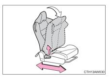
Lift the seatback angle adjustment lever.
