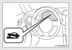
The hill-start assist control ON indicator will be illuminated when system is enabled and flash while the system is operating.
