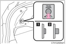
Turn the main switch in the trunk off to disable the trunk opener.
