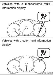
A diagnostic system continually monitors the readiness of the SRS airbag system (including front seat belt pretensioners) while the vehicle is being driven. The SRS warning light will show normal system operation by illuminating for approximately 6 seconds when the engine switch is turned to the "ON" position (vehicles without a smart key system), or the "ENGINE START STOP" switch is turned to IGNITION ON mode (vehicles with a smart key system).
