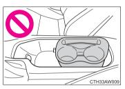
When placing the cup holder, make sure it is facing the correct direction. Failure to do so will cause the cup holder to not be secure in the console tray and hinder shift lever operation.
