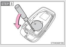
Remove the depleted battery.
