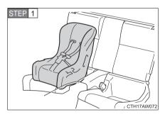
Place the child restraint system on the seat facing the front of the vehicle.
