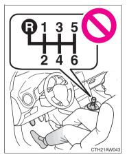
Do not shift the shift lever without depressing the clutch pedal.
