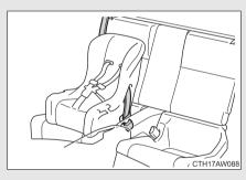
Seat belts equipped with a child restraint locking mechanism (ALR/ELR belts except driver's seat belt) (→P. 60)
