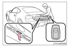
Press the button to unlock the trunk.
