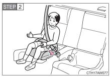
Sit the child in the child restraint system. Fit the seat belt to the child restraint system and insert the plate into the buckle. Make sure that the belt is not twisted.
