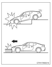
Only the driver's SRS frontal airbag or both driver's and front passenger's SRS frontal airbags may be activated when the vehicle sustains a hard impact in the undercarriage area from the road surface (such as when the vehicle plunges into a deep ditch, is severely impacted or knocked hard against an obstacle on the road such as a curb).
