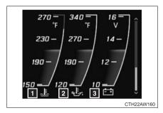
■ Engine coolant temperature gauge
