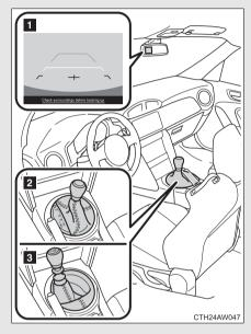
The rear view image will be displayed on the rear view monitor within a few seconds after the shift lever is shifted to R.
