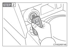
Touch the Toyota emblem side of the electronic key to the "ENGINE START STOP" switch.
