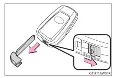
To take out the mechanical key, slide the release lever and take the key out.
