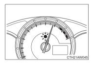
When the set engine speed is reached the RFV indicator comes on and a buzzer. sounds to inform the driver.
