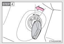
Vehicles without a smart key system: Stop the engine by turning the engine switch to the "ACC" position.
