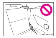
Always make sure that the seat belt is not caught in the seatback or twisted in one of the hooks that secure the seatback. Failure to do so may cause the seat belt to not be fastened correctly or to become ineffective in a collision, resulting in death or serious injury.
