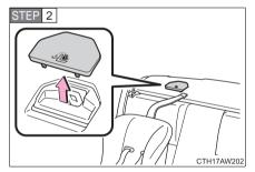
Remove the anchor bracket cover.
