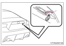
Turn the mechanical key clockwise to open.
