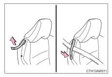
To enable the seat belt to be easily extended, pass the seat belt through the guide.
