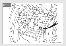
Remove the fuse with the pullout tool.
