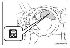
The slip indicator light will flash while the TRAC (brake LSD function)/VSC systems are operating.
