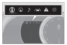
Selecting a menu icon displays a variety of vehicle data or allows vehicle settings to be customized.
