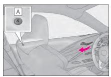
Pull the inside door handle to unlock the door.
