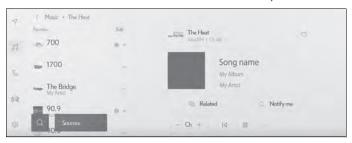
[Ch]: Touch [-]/[+] to search for the receivable channels. Touch and hold to switch channels. When released, the current channel is received.
