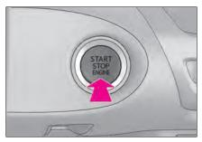
4 To stop the engine <a href="https://www.npress and hold the engine switch opening switch opening switch opening switch opening switch opening switch or 2 consecutive seconds or more, or press it briefly 3 times or more in succession.
