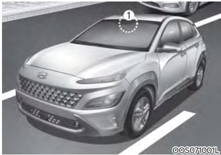
[1] : Front view camera (if equipped)
