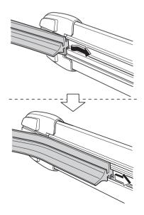
7. After pulling the blade rubber in the direction of the arrow and sliding the blade rubber to a position to check the blade holder groove, slide the blade rubber end in the opposite direction.
