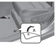
When setting a floor mat, position the floor mat so that its grommets are inserted over the pointed end of the retention posts.
