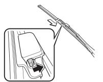
4. Pull the blade rubber in the direction of the arrow and slide it to a position where the blade holder groove can be checked.
