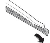
5. Remove the metal stiffeners from the blade rubber and install them in the new blade.
