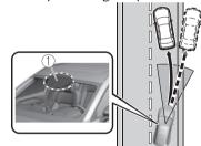
1. Forward sensing camera (FSC)
