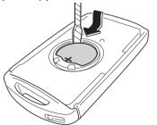
7. Insert a new battery into the transmitter so that the positive pole is facing up.
