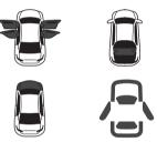
The light turns on if any door/liftgate/ hood is not closed securely.
