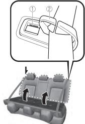
2. Press the seatback rearward and lock it in place. After returning the seatback to its upright position, make sure it is securely locked.
