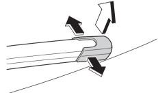
2. Remove the stopper and raise the wiper arm.
