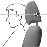
To raise a head restraint, pull it up to the desired position.
