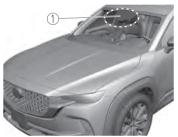
1. Forward Sensing Camera (FSC)
