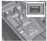
2. While checking the list displayed in the instrument cluster, push the Mi-Drive switch forward or pull it toward you to select a drive mode. Trailer is not connected
