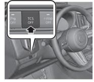
Press the switch again to turn the TCS back on. The TCS OFF indicator light<sup>\*</sup> will turn off.
