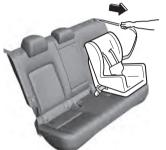
5. Push the child-restraint system firmly into the vehicle seat. Be sure the belt retracts as snugly as possible. A clicking noise from the retractor will be heard during retraction if the system is in the automatic locking mode. If the belt does not lock the seat down tight, repeat this step.
