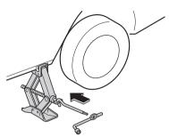
7. Turn the jack handle clockwise and raise the vehicle high enough so that the spare tire can be installed. Before removing the lug nuts, make sure your Mazda is firmly in position and that it cannot slip or move.
