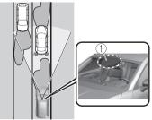
1. Forward Sensing Camera (FSC)<sup>\*1</sup>
