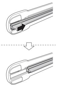
5. Pull the end of the blade rubber from the blade holder groove in the direction of the arrow and remove
