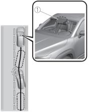
1. Forward sensing camera (FSC)
