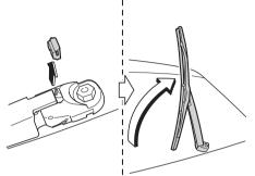
3. Firmly rotate the wiper blade to the right until it unlocks, then remove the blade.
