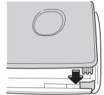
10.Insert the tabs of the lower cover into the slots of the transmitter and install the lower cover.
