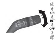
Turn the wiper on by turning the rear wiper/washer switch.
