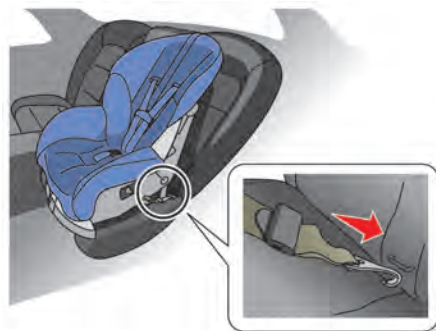
Forward-facing web-mounted — step 2
