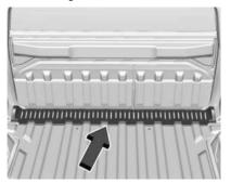
The midgate drain grate is located near the base of the midgate.
