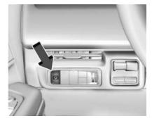
The Electric Parking Brake (EPB) can always be applied, even if the vehicle is off. In case of insufficient electrical power, the EPB cannot be applied or released. To prevent draining the battery, avoid unnecessary repeated cycles of the FPB
