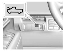
To open the hood, press the hood button on the instrument panel to the left of the steering wheel.
