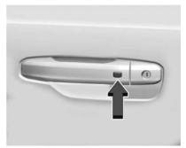
The remote key must be within 1 m (3 ft) of the eTrunk or door being opened or locked. Press the button on the door handle to open. See "Keyless Access Operation" in *Remote Key Operation*
