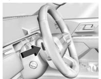
If equipped, Regen on Demand increases deceleration by pressing and holding the steering wheel paddle. Regen on Demand works in D (Drive). The accelerator pedal can be used to manage deceleration while using Regen on Demand. See One-Pedal Driving
