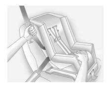
To tighten the belt, push down on the child restraint, pull the shoulder portion of the belt to tighten the lap portion of the belt, and feed the shoulder belt back into the retractor.
