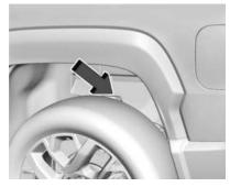
1. Reach around the tire to find the emergency manual charge cord release.
