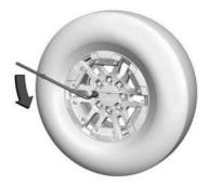
3. Turn the wheel wrench counterclockwise to loosen all the wheel nuts, but do not remove them yet.
