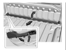
Keep the drain grate clean to avoid blocking the path of water to the gutter system. After hauling dirt, wood chips, pebbles, etc., check the midgate drain to ensure the drain path is clear. The drain grate can be removed and flushed with water if necessary.
