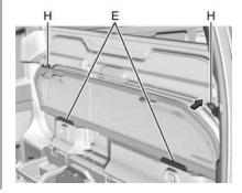
If equipped, open Corner Secures (H). Load the rear glass into the storage pocket in the midgate, guiding the lower edge of the rear glass behind the two rear glass retaining tabs (E).
