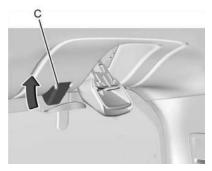
4. While holding the rear glass in place, press the glass-catch release button (C) and pull the top of the rear glass toward you using the grab handles (B) located at the top of the rear glass.
