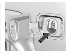
When the charge cord is plugged in, a color indicates the charging status.
