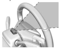
Sunglasses, hats, or other types of clothing that change the shape of the head may interfere with camera performance. To improve camera performance, raise or lower the steering wheel, wear lighter tinted glasses, or change the seat position.
