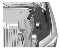
Complete a three-quarter turn on each of the three bolts and remove the right side access cover.
