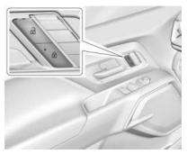
: Press to lock the doors. The indicator light in the switch will illuminate when locked.
