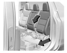
Pull the release strap located below the seat cushion to unlock the seatback. Fold the seatback forward and down.
