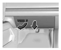
To open the glove box, pull the handle to the left. Use the mechanical key to lock or unlock. See Keys > 6.
