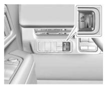
Rotate this thumbwheel to adjust the brightness of all illuminated controls. The thumbwheel is on the instrument panel to the left of the steering wheel.
