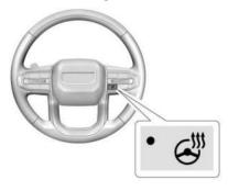
: Press to turn the heated steering wheel on or off. An indicator is lit when the feature is turned on.
