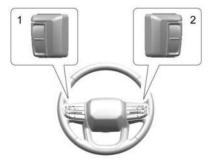
The favorites and volume switches are on the back of the steering wheel.
