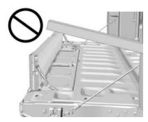
Do not place a load on top of the step when using it as a load stop.
