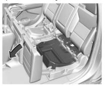
Pull the strap on the rear edge of the seat cushion to release. Tilt the seat cushion forward to access the storage. Rotate the seat bench rearward and push down to close.
