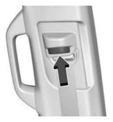
Push the release button to move the height adjuster to the desired position.
