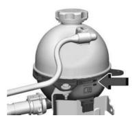
If the coolant level is not visible or needs to be adjusted within the reservoir, contact your dealer.
