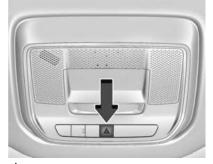
in Press this button on the overhead console to make the front and rear turn signal lights flash on and off. This warns others that you are having trouble. Press again to turn the flashers off.
