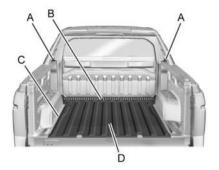
Even when all of these things are working properly and the cover system is on, there may be some instances (heavy rains, automated car washes, etc.) when water can collect in the following areas:
