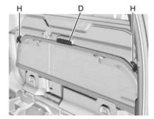
Push the glass against the glass stow retainer (D), located on the interior side of the door. Push until the glass handle slides down to lock the glass in place. If equipped, close corner secures (H).
