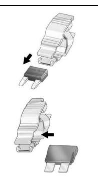
3. Use the fuse puller to remove the fuse from the top or side, as shown above.
