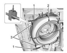
Lift the spare tire cage (2) slightly and manually disengage both hook ends (3).
