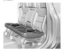
Pull the strap on the rear edge of the rear seat cushion to release the cushion. Tilt the seat cushion forward toward the front of the vehicle.
