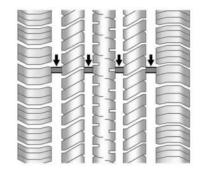
Treadwear indicators are one way to tell when it is time for new tires. Treadwear indicators appear when the tires have only 1.6 mm (1/16 in) or less of tread remaining. See *Tire Inspection* ⇔ 320 and *Tire Rotation* ⇔ 320.
