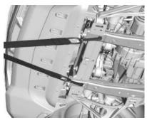
The vehicle is equipped with specific attachment points to be used to pull the vehicle onto a flatbed car carrier from a flat road
