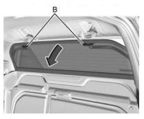
With the rear glass tilted toward you, lift it out from the lower window frame channel. Use the grab handles (B) to assist you in removing the rear glass.
