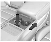
To access the floor console storage, press the cupholder button and slide the cupholders rearward.
