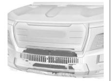
The vehicle may have a shutter system that automatically closes the frontal cooling openings. This system promotes airflow around the vehicle, reducing drag and providing energy savings. Ensure the shutter
