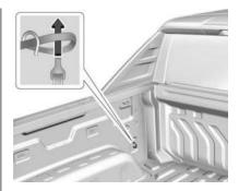
Place the loop end of the flat tire secure strap through the lower cargo tie-down on the driver side of the vehicle. Place the hook end of the strap through the loop and pull it until the strap is fastened securely to the tie-down.
