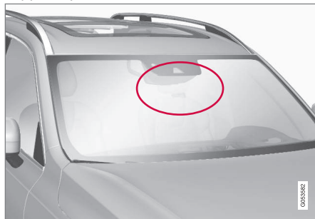
Location of radar sensor.
