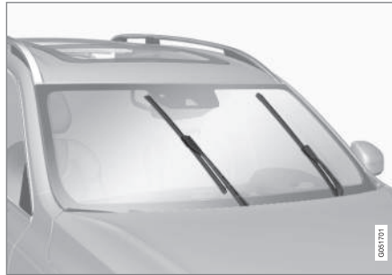
Windshield wipers in the service position.
