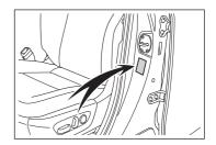
The gross vehicle weight must never exceed the GVWR indicated on the Certification Label.
