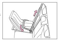
6 After installing the child restraint system, rock it back and forth to ensure that it is installed securely.
