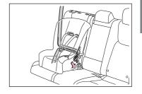
5 Fully extend the shoulder belt and allow it to retract to put it in lock mode. In lock mode, the belt cannot be extended.
