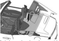
2. Switch your hand on the rear side of the front roof to the front side and pull the front roof forward.
