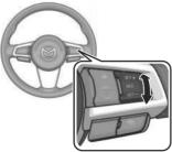
Constant speed driving starts when the vehicle speed is set. In addition, the set speed is displayed on the screen, and the MRCC standby indication (white) changes to the MRCC set indication (green) .
