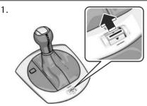
When the sport mode is selected, the select mode indicator light **SPORT** turns on in the instrument cluster.
