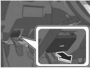
2. Insert your hand into the hood opening, slide the latch lever in the direction of the arrow as shown in the illustration, and lift up the hood
