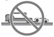
➤ Do not tow with sling-type equipment. This could damage your vehicle. Use wheel-lift or flatbed equipment.
