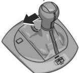
The gear position can be switched manually in manual shift mode. The manual shift mode indication and the gear position are displayed in the instrument cluster.
