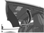
13.Install the headliner to the front roof using the fasteners at two locations.
