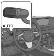
The HBC determines the surrounding conditions and operates automatically. When the HBC operates, the HBC indicator light (green) (in the instrument cluster turns on.
