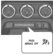
If the passenger occupant classification sensor is normal, the indicator light turns on when the ignition is switched ON. The light turns off after a few seconds. Then, the indicator light turns on or is off under the following conditions:
