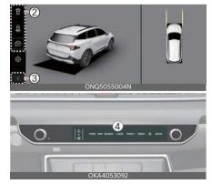
3D view function shows the vehicle in various angles. Press the 3D view icon
