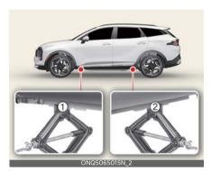
9. Insert the jack handle into the jack and turn it clockwise, raising the vehicle until the tire just clears the ground. This measurement is approximately 30 mm (1.2 inches). Before removing the wheel lug nuts, make sure the vehicle is stable and that there is no chance for movement or slippage.
