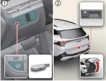
Press the power liftgate open/close button for 1 second. The liftgate opens or closes with a warning sound.
