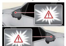
The warning light on the cluster, outside rearview mirror (side-view mirror) and head-up display (if equipped) will appear when the vehicle on both lanes is detected from the rear.
