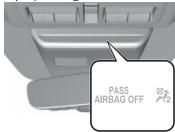
If the front passenger weight sensors are normal, the indicator light illuminates when the vehicle power is switched ON. The light turns off after a few seconds. Then, the indicator light illuminates or is off under the following conditions:
