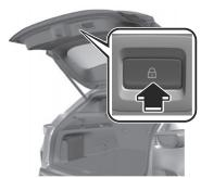
The following locations are locked by pressing the door-lock switch.
