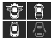
The light turns on if any door/liftgate/hood is not closed securely. In addition, the warning sound is activated if any door/trunk lid/liftgate is not closed and the vehicle is driven.
