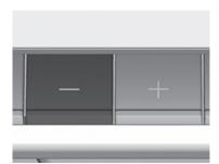
The airflow amount changes each time the switch is pressed. The airflow amount is indicated on the display. The airflow amount can be adjusted to 7 levels.
