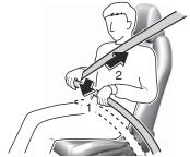
The belt should not touch the neck, jaw, or face and it should pass over the shoulder.
