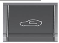
The mode is switched between recirculate mode and fresh air mode each time the switch is pressed. The display indicates whether recirculate mode (((a)) or fresh air mode ((a)) is selected.
