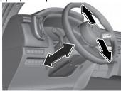
3. Pull up the lever to securely lock the steering wheel.
