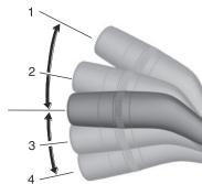
While the lever is in the 2 or 3 position, each turn signal light flashes and the turn signal light in the instrument cluster flashes. If you move the lever to the 2 or 3 position and release it immediately, the three-flash turn signal operates and the turn signal light flashes 3 times.
