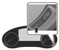
If you press the - switch again while the dashboard illumination is at maximum dimness, a sound is activated to notify you that the dimmer setting is at maximum dimness.
