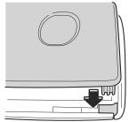
10.Attach the lower cover so that its tabs are inserted into the slots of the key.
