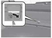
The liftgate is unlocked. After performing this emergency measure, have the vehicle inspected by an Authorized Mazda Dealer.
