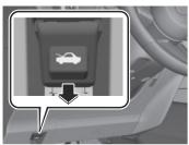
Insert your hand into the hood opening, slide the latch lever in the direction of the arrow as shown in the illustration, and lift up the hood.
