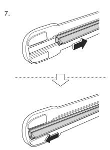
8. Make sure that the blade rubber is correctly installed to the blade holder.
