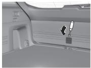
Move the lever. (Vehicles with power liftgate)
