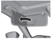
The visor extender\* extends the sunvisor's range of sun shading. To use, pull it out.
