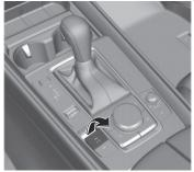
When the shift-linked release is enabled, a sound is activated 2 times, the EPB switch indicator light switches to fast flashing, and then flashes for a certain period of time.
