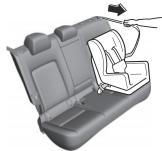
6. Push the child-restraint system firmly into the vehicle seat. Be sure the belt retracts as snugly as possible. A clicking noise from the retractor will be heard during retraction if the system is in the automatic locking mode. If the belt does not lock the seat down tight, repeat this step.
