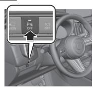
The parking sensors turn off and the parking sensor OFF switch indicator light turns on.
