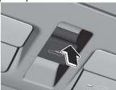
Press the tilt/slide switch forward 2 times.
