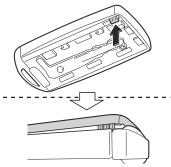
3. Insert a tape-wrapped flathead screwdriver into the gap and slide it.
