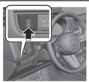
Press the i-ACTIVSENSE OFF switch to temporarily stop the following systems.
