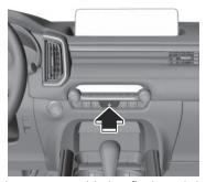
All the turn signal lights flash and the turn signal light in the instrument cluster flashes.
