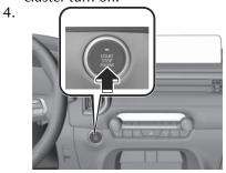
The engine starts and the KEY indicator light (green) <sup>∞</sup> in the instrument cluster turns off.
