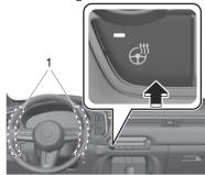
1. Heating area The indicator light in the heated steering wheel switch turns on.
