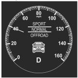
When the drive mode is set, the display in the instrument cluster changes.
