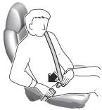
5. The belt should fit the pelvis as low as possible.
