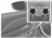
Press the adjustment switch to adjust the angle of the outside mirror.
