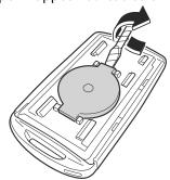
6. Remove the battery using the tape-wrapped flathead screwdriver.
