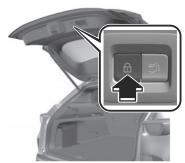
The doors, liftgate, and the fuel-filler lid are locked, the hazard warning lights operate 1 time.
