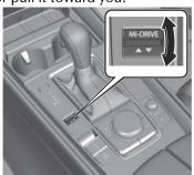
2. While checking the list displayed in the instrument cluster, push the Mi-Drive switch forward or pull it toward you to select a drive mode.
