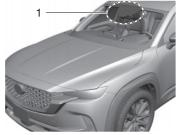
1. Forward Sensing Camera (FSC)
