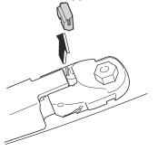
Raise the wiper arm and rotate the wiper blade to the right until it unlocks, then remove the blade.
