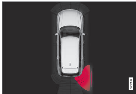
Illuminated Cross Traffic Alert icon in the Park Assist System graphic on the screen.
