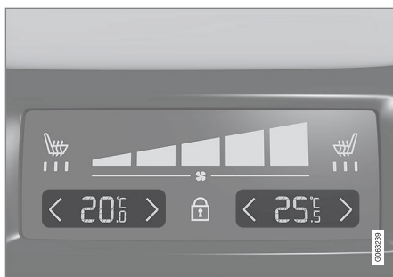
Temperature controls on the rear climate panel of the tunnel console.
