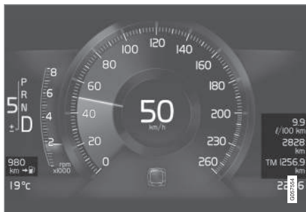
Example of trip computer information in an 8-inch instrument panel. The illustration is generic - details may vary according to vehicle model.
