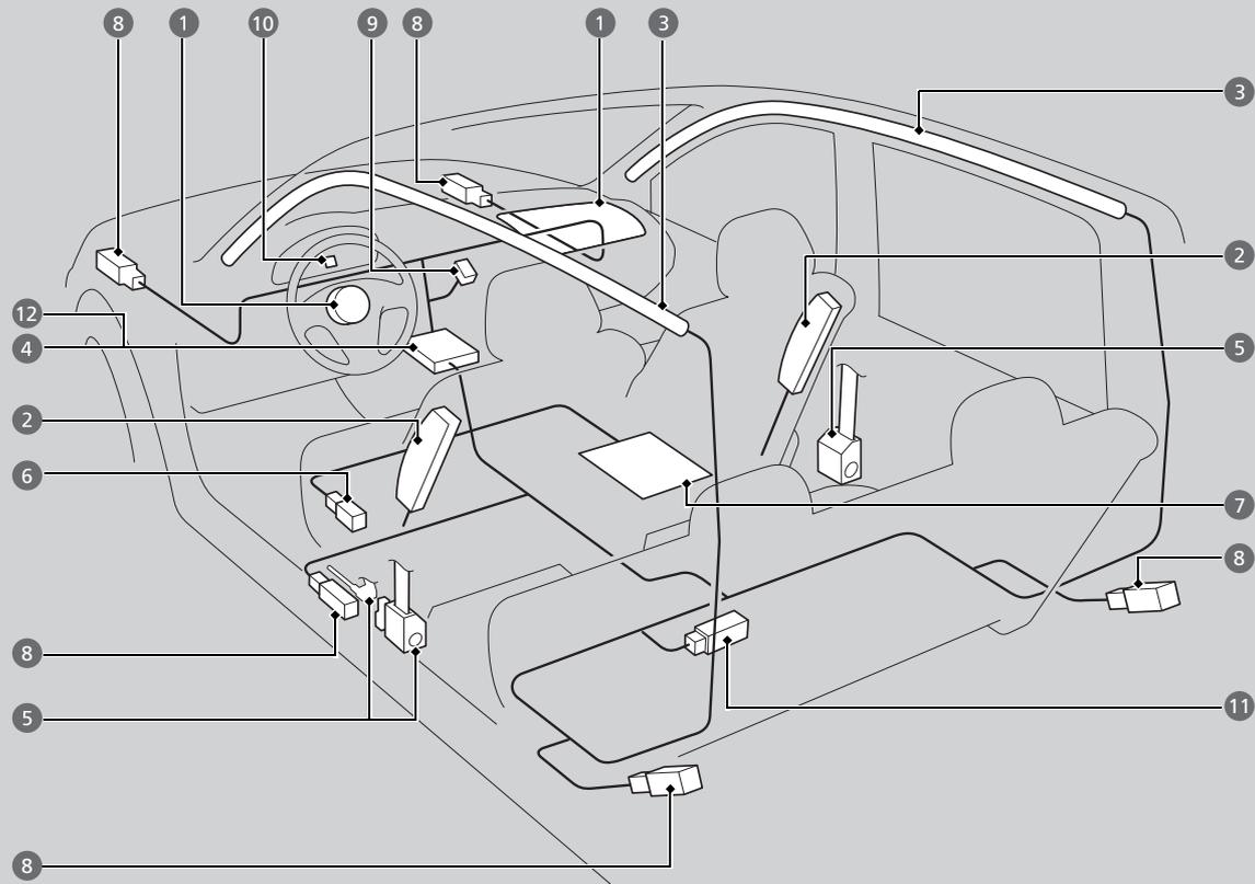
The front, side, and side curtain airbags are deployed according to the direction and severity of impact. Both side curtain airbags are deployed in a rollover. The airbag system includes:
