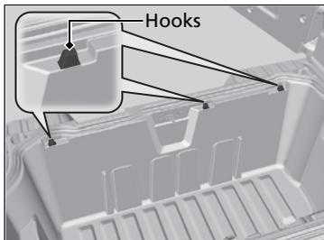
There are three hooks for plastic grocery bags at the back of the trunk. They are designed to hold light items. Heavy objects may damage the hooks.
