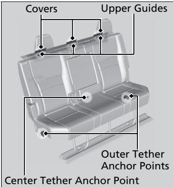
A tether anchor point is provided at each outside of the seat bottom and between the lower anchors of the rear center seat. If you have a child seat that comes with a tether but can be installed with a seat belt, the tether may be used for additional security.
