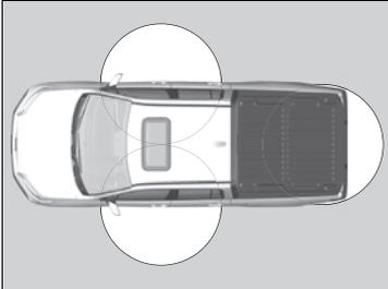
When you carry the keyless remote, you can lock/unlock the doors and open the trunk.
