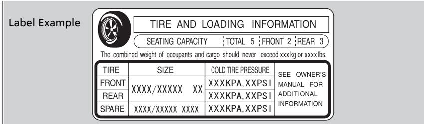
This figure includes the total weight of all occupants, cargo, and accessories, and the tongue load if you are towing a trailer.
