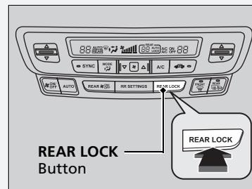
Press the **REAR LOCK** button to turn the rear lock mode on and off.
