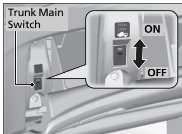
The trunk main switch disables the trunk release button on the trunk lid to protect luggage in the trunk.
