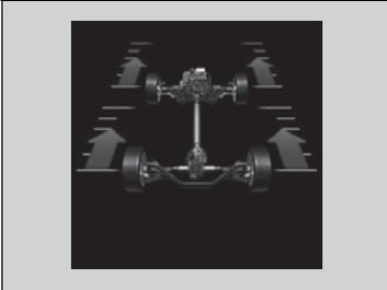
The indicators on the display show the amount of torque being transferred to the right front, left front, right rear, and left rear wheels.
