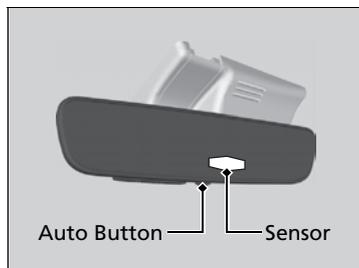
When you are driving after dark, the automatic dimming rearview mirror and power door mirrors\* reduce the glare from headlights behind you. Press the auto button to turn this function on and off. When activated, the auto indicator comes on.
