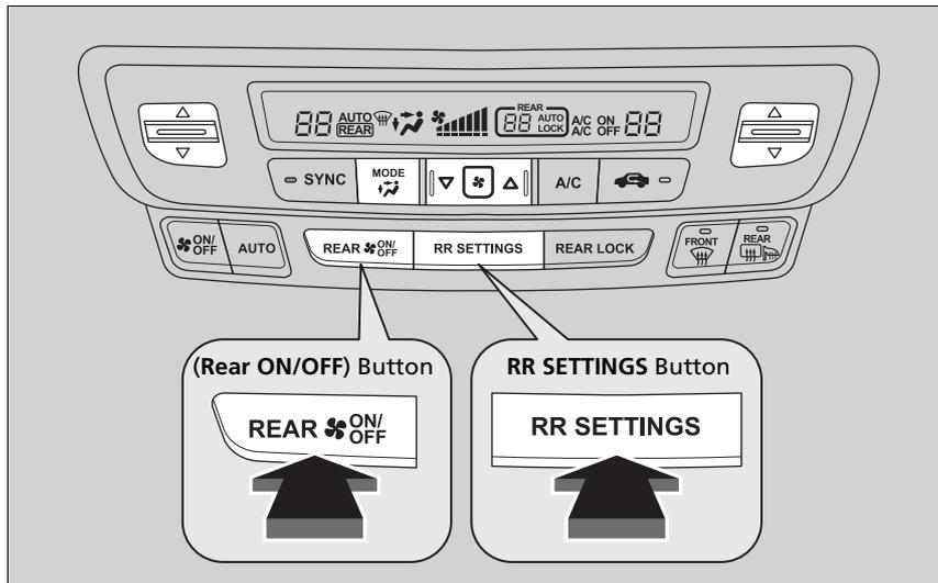
Use the system when the engine is running and the climate control system is operating.
