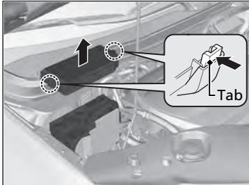
Located near the passenger's side damper house. Push the tabs to open the box. Fuse locations are shown on the fuse box cover. Locate the fuse in question by the fuse number and box cover number.
