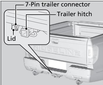
Open the lid of the socket (located next to the trailer hitch) to expose the 7-pin trailer connector.
