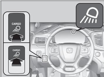
The bed lights can be turned on or off by pressing the button when the transmission is in **P**.
