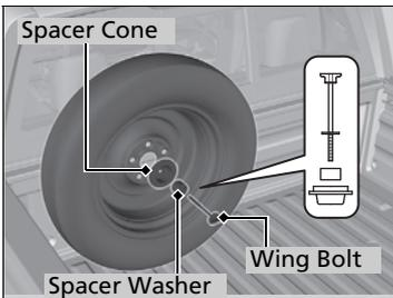
3. Place the compact spare tire on the pickup bed as shown.
