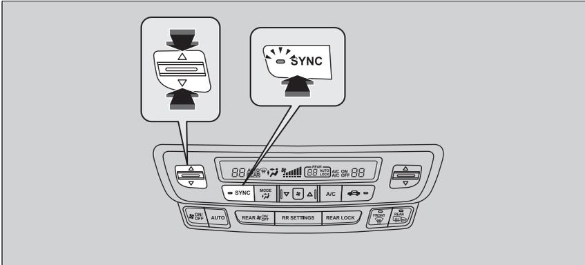
You can set the temperature synchronously for the driver side, front passenger side and rear seats in synchronized mode.
