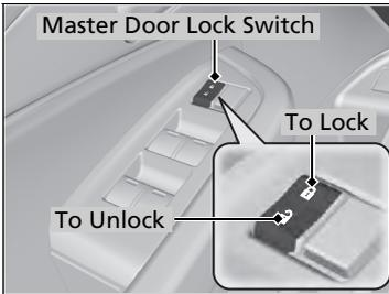
Press the master door lock switch in as shown to lock or unlock all the doors.
