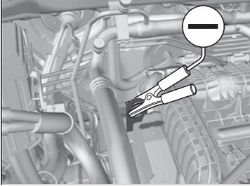
5. Connect the other end of the second jumper cable to the engine hanger as shown. Do not connect this jumper cable to any other part.
