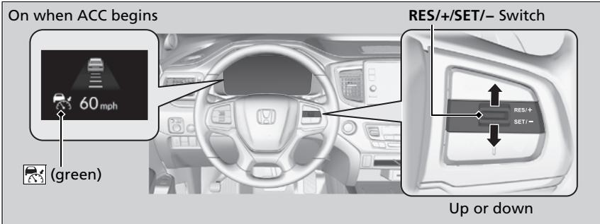
Take your foot off the pedal and press the **RES/+ / SET/-** switch up or down when you reach the desired speed. The moment you release the switch, the set speed is fixed, and ACC begins.
