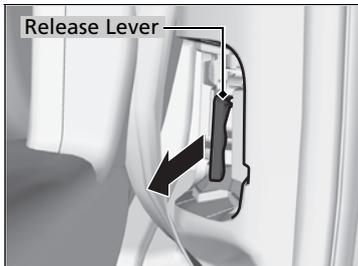
3. Pull the release lever as shown.
