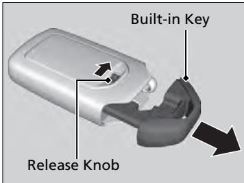
The built-in key can be used to lock/unlock the doors or open the trunk when the keyless remote battery becomes weak and the power door lock/unlock operation is disabled.
