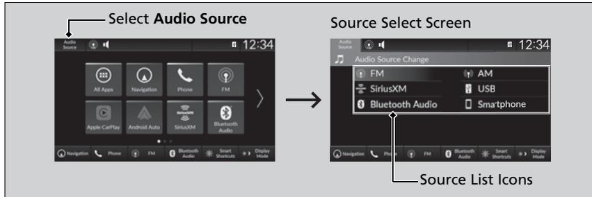
Select **Audio Source** in the header area, then select an icon on the source list to switch the audio source.
