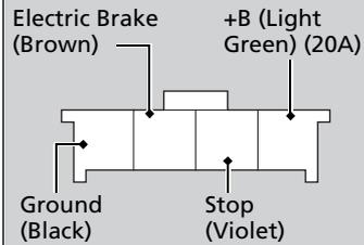
Have a qualified mechanic install your trailer brake controller following the trailer brake controller manufacturer's instructions. Failure to properly install the trailer brake controller may increase the distance it takes for you to stop your vehicle when towing a trailer.
