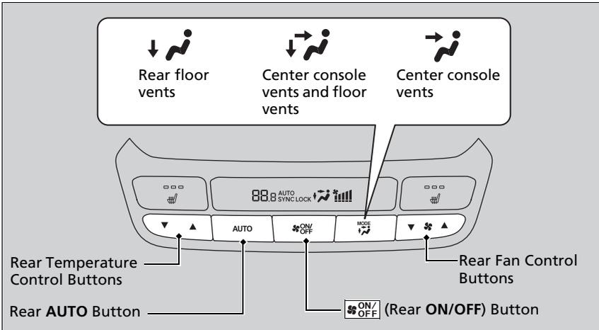
Use the system when the engine is running and the climate control system is operating.
