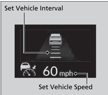
When ACC starts operating, the vehicle icon, interval bars and set speed appear on the driver information interface.
