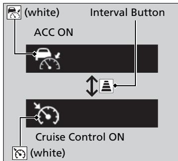
Press and hold the Interval button for one second. **Cruise mode selected** appears on the driver information interface for two seconds, and then the mode switches to Cruise.
