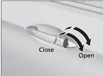
**To open:** Unlock the driver's door with the key. Within 10 seconds of returning the key to the central position, turn the key in the unlock direction and hold it there.
