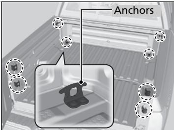
The tie-down anchors on the pickup bed can be used to install a net for securing items.
