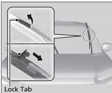
2. Using a flat-tip screwdriver, pry up on the edge of the lock tab to release it. Wrap the flat-tip screwdriver with a cloth to prevent scratches.
