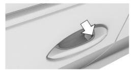
Touch the grooved surface on the handle of a closed vehicle door with your finger for approx. 1 second without grasping the door handle.
