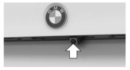
The camera is located in the handle of the trunk lid.
