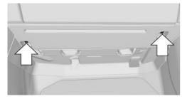
Loosen fasteners, arrows, and open cover.
