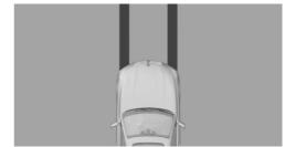
The car wash view assists when entering a car wash by displaying the floor and the vehicle's own track.
