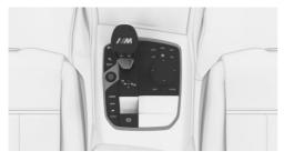
Press the rocker switch repeatedly until the desired program is displayed in the instrument cluster.
