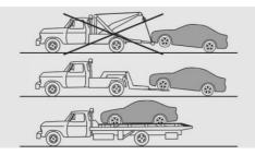
Your vehicle should be transported with a tow truck with a so-called lift bar or on a flat bed.
