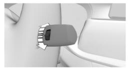
Turn the thumbwheel on the wiper lever.
