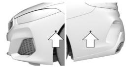
The ultrasound sensors of the Automatic Parking Assistant are located on the side of the vehicle.
