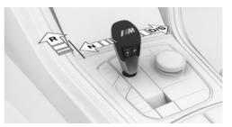
With the driver's safety belt fastened, press on the brake pedal and pull or push the selector lever in the required direction. The selector lever automatically returns to the center position when released.
