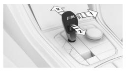
Push the selector lever out of Drive mode in the D/S direction, arrow 1, or shift via the selector lever, arrows at 2.
