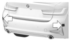
The radar sensors are located in the bumper.
