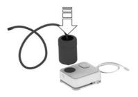
Screw the filler hose of the sealant bottle onto the tire valve of the nonworking wheel.
