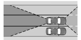
Radar sensors monitor the space next to the vehicle when traveling faster than a minimum speed of up to approx. 130 mph/210 km/h.
