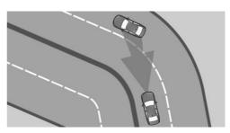
When you approach a curve the system may briefly report vehicles in the next lane due to the bend of the curve. If the system decelerates you may compensate it by briefly accelerating. After releasing the accelerator pedal the system is reactivated and controls speed independently.
