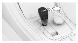
Push the selector lever out of the center position in the D/S direction.
