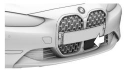
The radar sensor is located in the front bumper.
