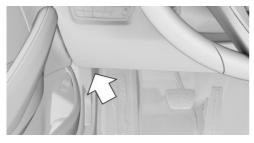
Located on the driver's side is an OBD socket for reading the vehicle data.
