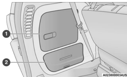
Vacuum System Access Panels
