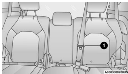
Routing The Rear Seat Belt Latch Plate
