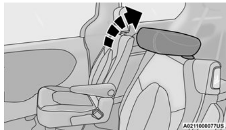
Fold Headrest To Upward Position
