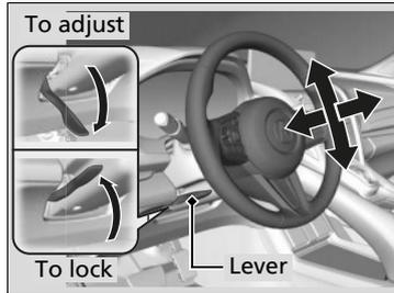
1. While the vehicle is stopped, push the steering wheel adjustment lever down.
