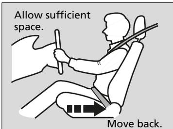
Adjust the driver's seat as far back as possible while allowing you to maintain full control of the vehicle. You should be able to sit upright, well back in the seat and be able to adequately press the pedals without leaning forward, and grip the steering wheel comfortably. The passenger's seat should be adjusted in a similar manner, so that it is as far back from the front airbag in the dashboard as possible.
