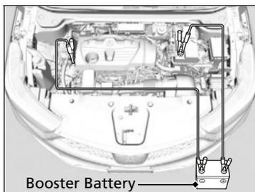
1. Open the fuse box cover on your vehicle's 12-volt battery positive  $\oplus$  terminal.
