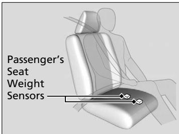
The front passenger's advanced airbag system has weight sensors. The sensors are used for occupant classification to activate or deactivate the front passenger's airbag.
