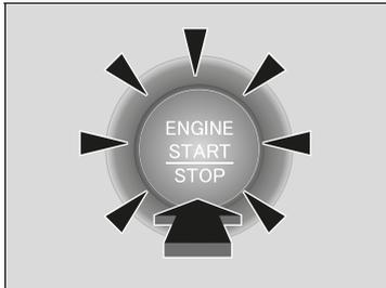
1. Touch the center of the **ENGINE START/STOP** button with the **A** logo on the keyless remote while the **ENGINE START/STOP** button is flashing. The buttons on the keyless remote should be facing you.
