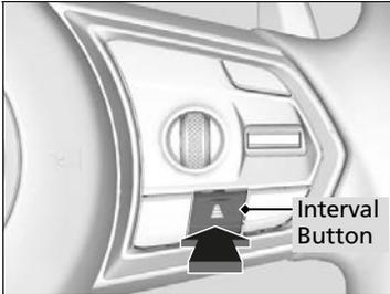
Press the interval button to change the ACC with Low Speed Follow following-interval. Each time you press the button, the following-interval (the interval behind a vehicle detected ahead of you) setting cycles through extra long, long, middle, and short following-intervals.
