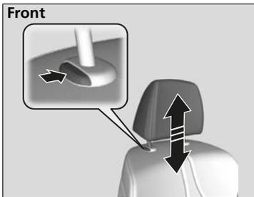
**To raise the head restraint:** Pull it upward.
