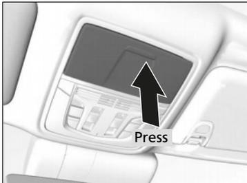
To open the sunglasses holder, press and release the indent. To close, press it again until it latches.
