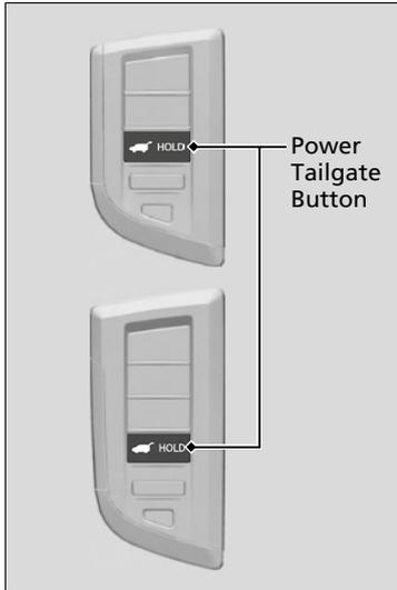
Press the power tailgate button for more than one second to operate when the power mode is in VEHICLE OFF (LOCK).
