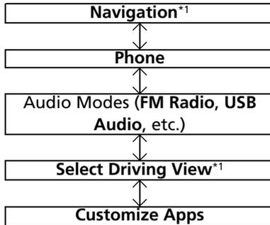
After an audio mode is selected, the left selector wheel can be operated for the following functions.
