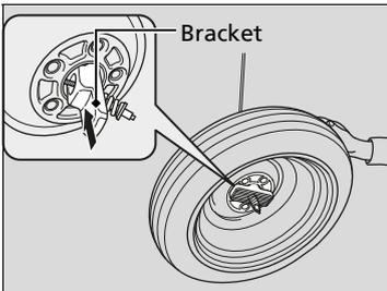
**6.** Keep turning the wheel nut wrench to create slack in the cable.
