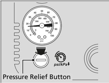
11. Press the pressure relief button until the gauge returns 0 psi (0 kPa).
