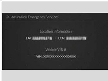
If your vehicle's airbags deploy or if the unit detects that the vehicle is severely impacted, your vehicle automatically will attempt to connect to the AcuraLink operator. If connected, information about your vehicle, its location, and its condition can be sent to the operator\*1; you also can speak to the operator when connected.
