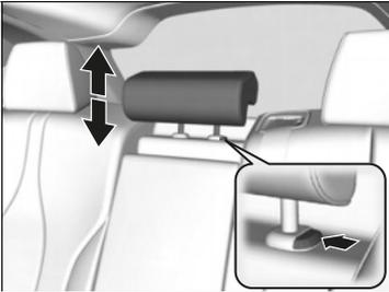
A passenger sitting in a center back seating position should adjust the height of their head restraint to an appropriate position before the vehicle begins moving.
