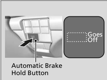
While the system is on, press the automatic brake hold button again.
