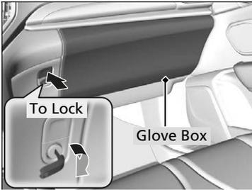
Press the button to open the glove box. You can lock the glove box with the built-in key.
