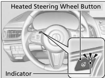
The power mode must be in ON to use the heated steering wheel.
