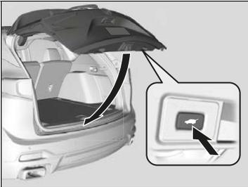
Press the button on the tailgate to close the power tailgate.
