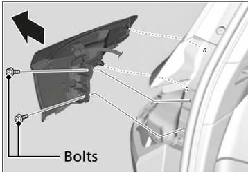
2. Use a Phillips-head screwdriver to remove the bolts.
