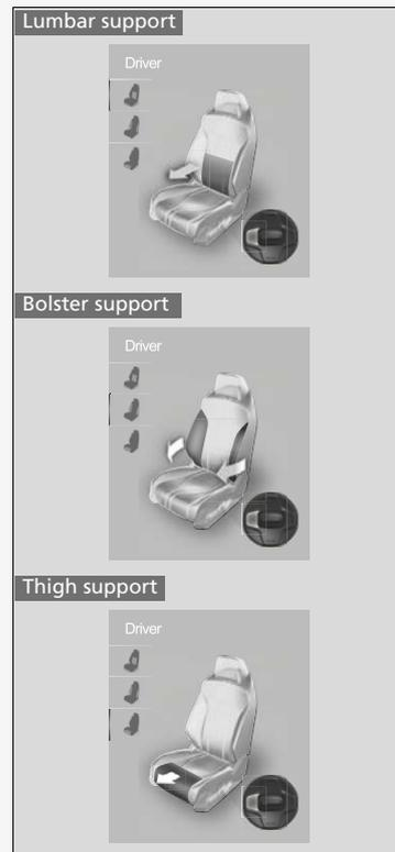
1. Press the mode selector up or down to select the lumbar support adjustment mode, bolster support adjustment mode or thigh support adjustment mode.
