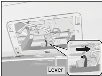
2. To open the tailgate, push the tailgate while sliding the lever to the right.
