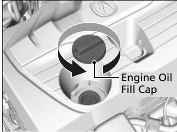
1. Unscrew and remove the engine oil fill cap.
