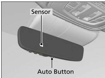
When you are driving after dark, the automatic dimming rearview mirror and automatic dimming power door mirrors reduce the glare from headlights behind you, based on inputs from the mirror sensor. Press the auto button to turn this function on and off. When activated, the auto indicator comes on.
