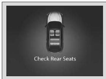
A reminder appears on the multi-information display and an alert will sound when the power mode is set to VEHICLE OFF.
