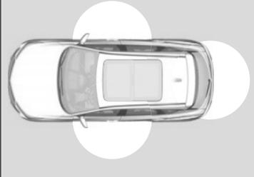
When you carry the keyless remote, you can lock/unlock the doors and fuel fill door, and open the tailgate.
