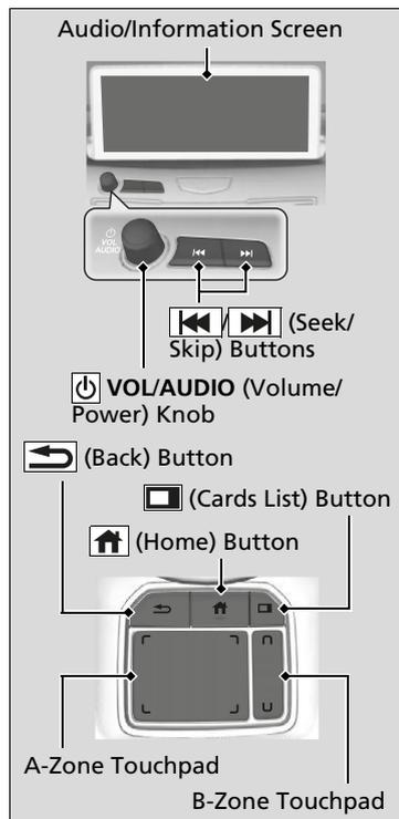
**VOL/AUDIO (Volume/Power) Knob:** Push to turn the audio system on and off. Turn to adjust the volume when the audio system is on.
