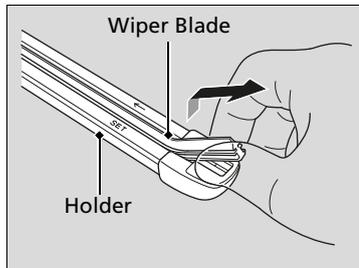
**6.** Pull the wiper blade in the opposite direction to slide it out of the holder.
