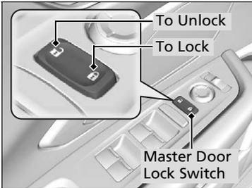
Press the master door lock switch in as shown to lock or unlock all the doors, tailgate and fuel fill door.
