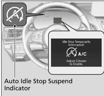
The Auto Idle Stop suspend indicator comes on and a message appears on the multi-information display. when the Auto Idle Stop system cannot be activated.
