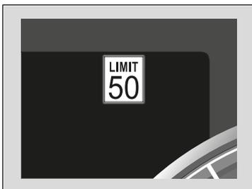
Shows the current speed limit based on either information compiled through the navigation system\* or speed limit signs captured by the front sensor camera.
