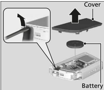
2. Pry on the edge of the cover using a flat-tip screwdriver to remove the cover.
