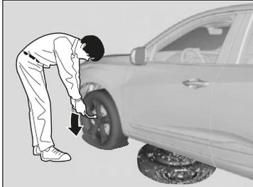
**10.** Loosen each wheel nut about one turn using the wheel nut wrench.
