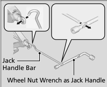
3. Raise the vehicle, using the jack handle bar and the jack handle, until the tire is off the ground.
