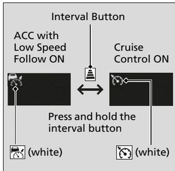
Press and hold the interval button for one second. **Cruise Mode Selected** appears on the multi-information display for two seconds, and then the mode switches to Cruise.
