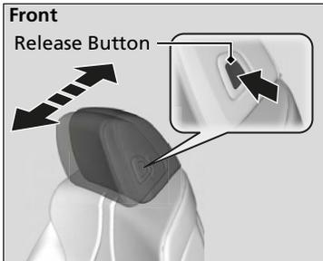
**To adjust the front head restraint forward:**
