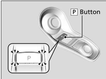
Park your vehicle in a safe place with the power mode in ON, then apply the brakes and press the **P** button to put the transmission in Park.
