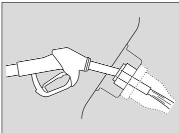
6. Place the end of the filler nozzle on the lower part of filler opening, then insert it slowly and fully.
