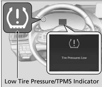
Monitors the tire pressure while you are driving. If your vehicle's tire pressure becomes significantly low, the low tire pressure/TPMS indicator comes on and a message appears on the multi-information display.
