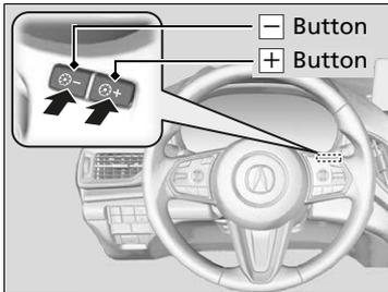
When the power mode is in ON, you can use the **+** or **-** button to adjust instrument panel brightness.
