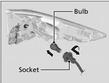
4. Turn the socket counterclockwise and remove it.
