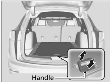
1. Push the rear edge of the handle on the floor lid and open the lid.
