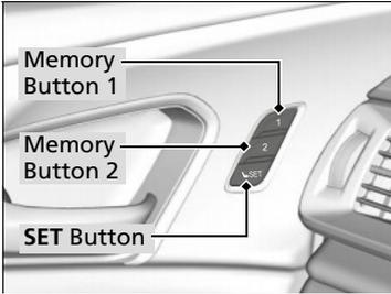
1. Set the power mode to ON. Adjust the driver's seat and the door mirrors to the desired position.
