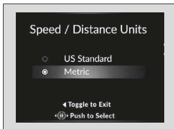
Enables you to show another unit on the multi-information display, head-up display\* and audio/information screen and set the displayed measurements to read in either miles and mph or km and km/h.
