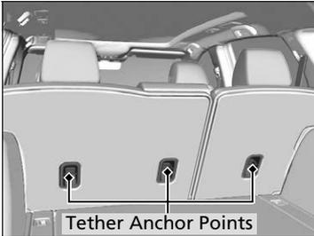
A tether anchor point is provided behind each rear seating position.
