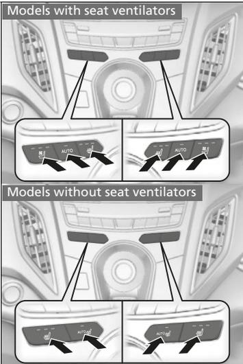
Press the seat heater or the seat ventilator\* button:
