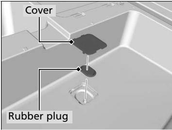
**4.** Remove the cover and the rubber plug on the cargo area lining to access the shaft for the spare tire hoist.
