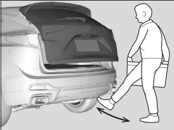
Use a forward and back kicking motion for about 1 second under the center of the rear bumper to open or close the power tailgate while carrying the keyless remote.
