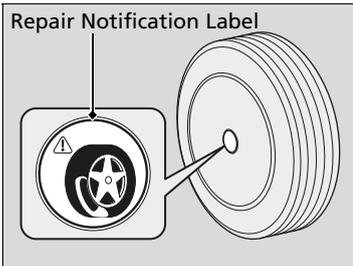
12. Apply the repair notification label to the flat surface of the wheel.
