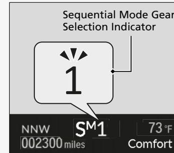
The transmission is in **S** and **Sport** mode, to prioritize the engine performance enhancement, the transmission may not allow for shifting up while the engine speed is low.
