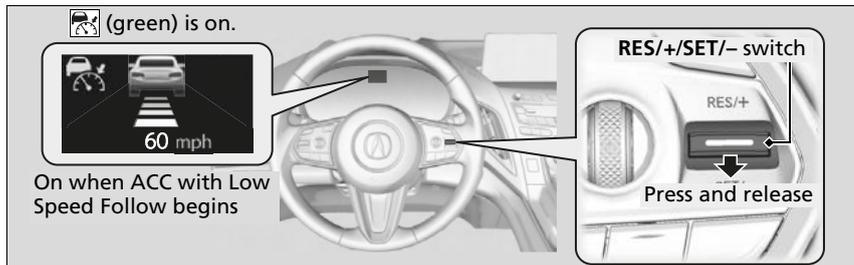
**When driving at about 25 mph (40 km/h) or above:** Take your foot off the pedal and press down the **RES/+ / SET / -** switch when you reach the desired speed. The moment you release the switch, the set speed is fixed, and ACC with Low Speed Follow begins.
