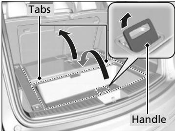
Pull the handle and remove the tabs to open the cargo floor lid.
