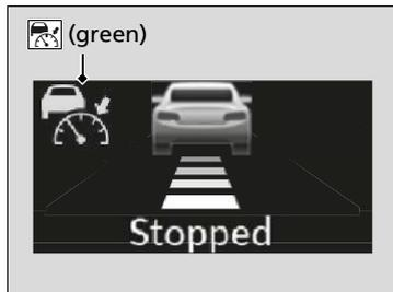
Your vehicle also stops, automatically. The **Stopped** message appears on the multi-information display. When the vehicle ahead of you starts again, the vehicle icon on the multi-information display blinks. If you press the **RES/+ / SET / -** switch up or down, or depress the accelerator pedal, ACC with Low Speed Follow operates again within the prior set speed.
