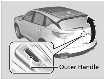
When all the doors are unlocked, the tailgate is unlocked.
