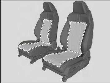
The seat heaters or ventilators\* can be used when the power mode is in ON.
