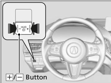
When the power mode is in ON, you can use the **+**/**-** button to adjust head-up display brightness.
