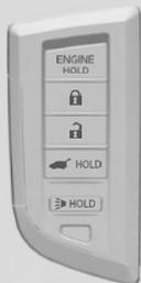
Use the keys to start and stop the engine, lock and unlock all the doors and the fuel fill door, and open the tailgate.
