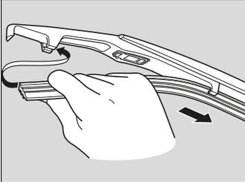
4. Slide the new wiper blade onto the holder.
