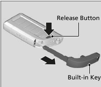
The built-in key can be used to lock/unlock the doors when the keyless remote battery becomes weak and the power door lock/unlock operation is disabled.
