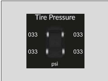
To select the tire pressure monitor, set the power mode to ON, and roll the right selector wheel until you see the tire pressure screen.
