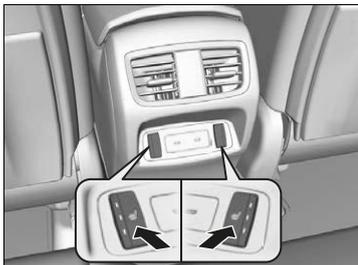
The seat heaters can be used when the power mode is in ON.
