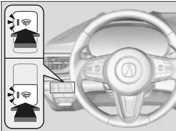
The heated windshield will automatically switch off after 15 minutes.
