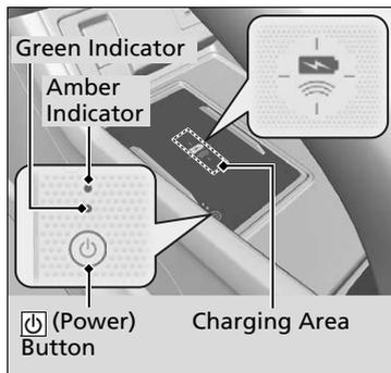
1. To turn the system on and off, press and hold the
