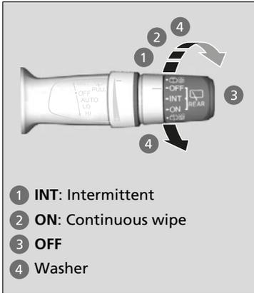
The rear wiper and washer can be used when the power mode is in ON.
