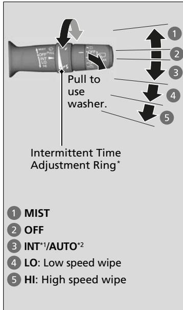
The windshield wipers and washers can be used when the power mode is in ON.
