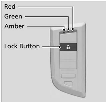
You can remotely check if your vehicle's doors are all locked or any are unlocked using the keyless remote from extended distances.
