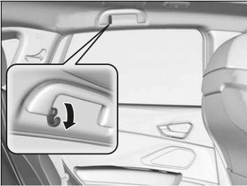
There are coat hooks on the rear grab handle of both sides. Pull it down to use it.
