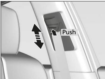
1. Move the anchor up and down while holding the release button.
