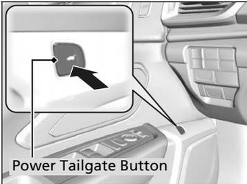
To open or close the power tailgate, press the power tailgate button for about one second.
