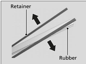
3. Remove the retainers from wiper blade and mount to a new rubber blade.
