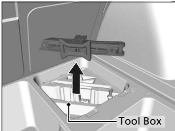
3. Take the jack, wheel nut wrench, and jack handle bar out of the tool box.
