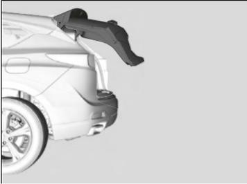
The extent to which the power tailgate automatically opens can be programmed.
