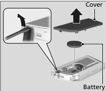
▶▶ Replacing the Remote Battery
