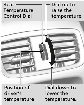
You can set the rear passenger compartment temperature different than the driver's, using the rear temperature control dial.
