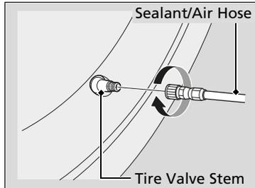
3. Attach the sealant/air hose onto the tire valve stem. Screw it until it is tight.
