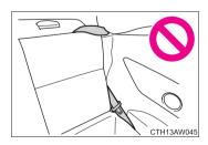
Always make sure that the seatbelt is not caught in the seatback or twisted in one of the hooks that secure the seatback. Failure to do so may cause the seatbelt to not be fastened correctly or to become ineffective in a collision. resulting in serious injury.
