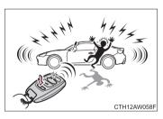
When ((\*) is pressed for longer than about one second, an alarm will sound intermittently and the vehicle lights will flash to deter any person from trying to break into or damage your vehicle.
