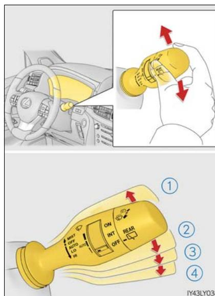
The sensor sensitivity can be adjusted when "AUTO" is selected.
