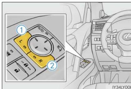
**2** To adjust the mirror, press the switch.
