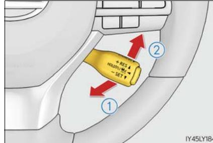
However, when a vehicle ahead is not detected, cruise control does not resume when the vehicle speed is approximately 25 mph (40 km/h) or less.
