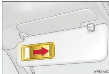
If the vanity lights remain on when the engine switch is turned off, the lights will go off automatically after 20 minutes.
