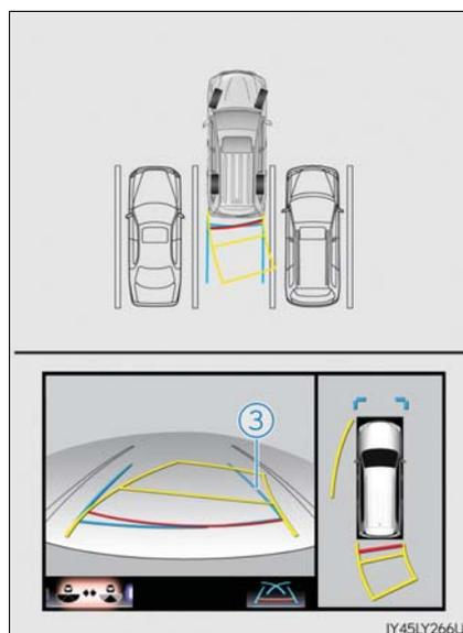
4 Once the vehicle width extension guide lines and the parking space lines are parallel, straighten the steering wheel and back up slowly until the vehicle has completely entered the parking space.
