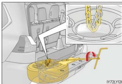
**4** Confirm that the tire is not loose after tightening:
