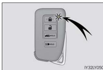
The smart access system with push-button start uses weak radio waves. In the following situations, the communication between the electronic key and the vehicle may be affected, preventing the smart access system with push-button start, wireless remote control and engine immobilizer system from operating properly. (Ways of coping: →P. 551)
