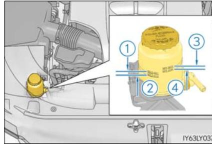
**Hot:** The vehicle has been driven around 50 mph (80 km/h) for 20 minutes, or slightly longer in frigid temperatures.
