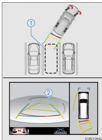
3 When the rear position of the vehicle has entered the parking space, turn the steering wheel so that the vehicle width extension guide lines are within the left and right dividing lines of the parking space.
