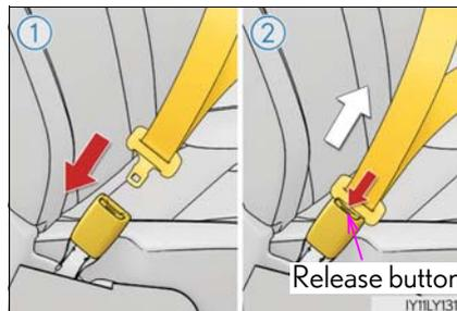
**Fastening and releasing the third center seat belt (if equipped)**
