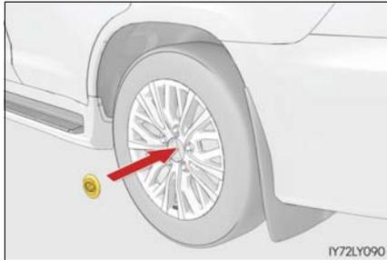
Remove the center wheel ornament from the flat tire by pushing from the reverse side, and reinstall it.
