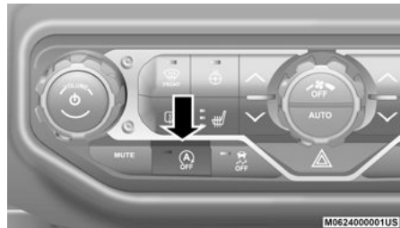
Stop/Start OFF Switch
