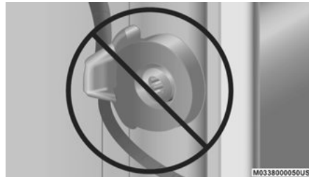
Incorrectly Seated Tailgate Strap
