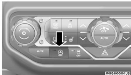
Stop/Start OFF Switch
