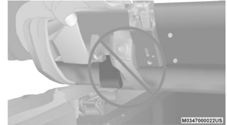
Incorrectly Seated Retainer
