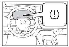
9 If the specified tire inflation pressure of the wheel set installed differs from that of the previous set, it will be necessary to perform the tire inflation pressure setting procedure of the tire pressure warning system. (→P.290)
