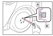
When replacing an aluminum wheel with a steel wheel, tighten the wheel nuts until the tapered portion A comes into loose contact with
