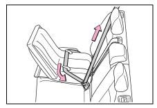
5 After installing the child restraint system, rock it back and forth to ensure that it is installed securely. (→P.55)
