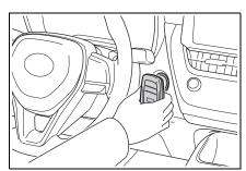
Firmly depress the brake pedal and check that is shown on the multi-information display. 4 Press the engine switch shortly and firmly.
