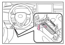
Remove the fuse with the pullout tool.
