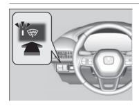
Press the heated windshield button to deice the windshield at the wiper park area of the windshield when the power mode is in ON.
