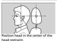
Head restraints are most effective for protection against whiplash and other rearimpact crash injuries when the center of the back of the occupant's head rests against the center of the restraint. The tops of the occupant's ears should be level with the center height of the restraint.
