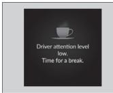
If one bar lights up, the **Driver attention level low. Time for a break.** message will appear, a beep will sound, and the steering wheel will vibrate.
