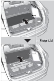
**1.** Fold the cargo area floor lid into three parts.
