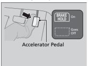
Depress the accelerator pedal while the transmission is in a position other than  $\boxed{\mathbf{P}}$  or  $\boxed{\mathbf{N}}$ . The system is canceled and the vehicle starts to move.
