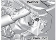
**4.** Remove the drain bolt and washer from the bottom of the engine, and drain the oil into a suitable container.
