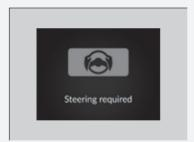
If the driver does not grip the steering wheel after the warning above has repeatedly appeared, a warning buzzer will sound and Traffic Jam Assist will be canceled.
