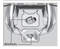
The tie-down anchors on the cargo area floor can be used to install a net for securing items.
