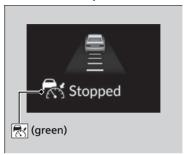
Your vehicle also stops, automatically. The **Stopped** message appears on the gauge. When the vehicle ahead of you starts again, if you press the **RES/+/SET/-** switch up or down, or depress the accelerator pedal, ACC with Low Speed Follow operates again within the prior set speed.
