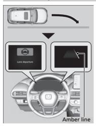
The front wide view camera behind the rearview mirror monitors left and right lane markings in white or yellow, the outer edge of the pavement (into grass or gravel road shoulder) or a detected oncoming vehicle. If your vehicle approaches any detected lane markings, the outer edge of the pavement (into grass or gravel road shoulder) or a detected oncoming vehicle when the turn signals have not been engaged, the system activates.
