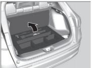
Fold the cargo area floor lid into three parts.
