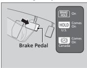
Depress the brake pedal to come to a complete stop. The transmission must not be in  $\boxed{\mathbf{P}}$  or  $\boxed{\mathbf{R}}$ .
