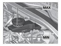
The fluid level should be between the **MIN** and **MAX** marks on the side of the reserve tank.
