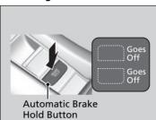
Only the automatic brake hold system indicator comes on:
