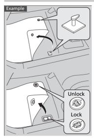
The driver's floor mat hooks over the floor anchors, which keep the mat from sliding forward.
