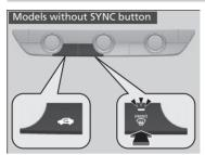
Pressing the button turns the air conditioning system on and automatically switches the system to fresh air mode.
