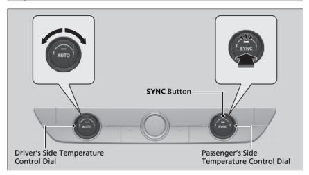
You can set the temperature synchronously for the driver's side and the passenger's side in synchronization mode.
