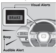
The system provides visual and audible alerts of a possible collision, and stops if the collision is avoided.
