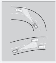
When the vehicle ahead of you moves away, such as when entering an interchange or rest area, ACC with Low Speed Follow may continue to maintain the set following-interval for a short time.
