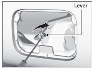
**2.** To open the tailgate, push the tailgate while sliding the lever to the right with the flat-tip screwdriver.
