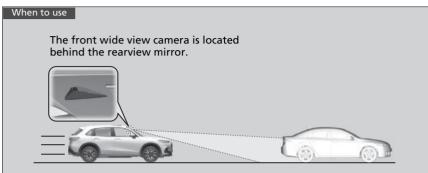
The system starts monitoring the roadway ahead when your vehicle speed is about 3 mph (5 km/h) or above and will search for a vehicle (including motorcycles), pedestrian, or moving bicycle in front of you.
