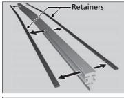
**4.** Remove the retainers from the rubber blade that has been removed, and mount to a new rubber blade.
