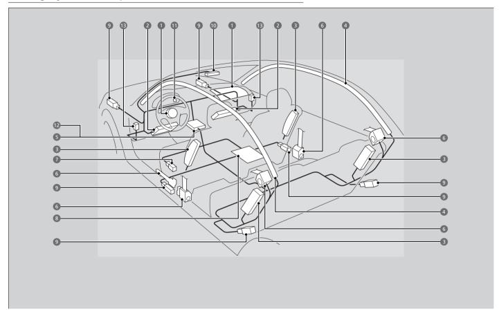
The front, driver's knee, front passenger's knee, side, and side curtain airbags are deployed according to the direction and severity of impact. Both side curtain airbags are deployed in a rollover. The airbag system includes:
