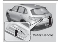
When all the doors are unlocked or press the tailgate unlock button on the remote transmitter, the tailgate is unlocked. Press the tailgate outer handle and lift open the tailgate.
