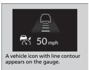
Your vehicle maintains the set speed without having to keep your foot on the brake or accelerator pedal.
