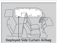
The side curtain airbag is designed to deploy in a rollover or a moderate-to-severe side impact.
