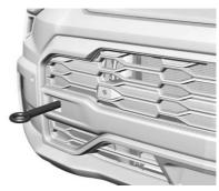
The vehicle is equipped with a tow eye. Only use the tow eye to pull the vehicle onto a flatbed car carrier from a flat road surface. Do not use the tow eye to pull the vehicle from snow, mud, sand, or ditch.
