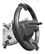
To adjust the steering wheel, if equipped:
