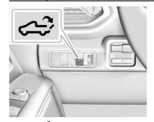
Press on the instrument panel to the left of the steering wheel.
