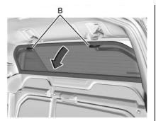
With the rear glass tilted toward you, lift it out from the lower window frame channel. Use the grab handles (B) to assist you in removing the rear glass.
