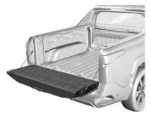
• Press 📆 twice quickly on the remote key until the tailgate moves. See Remote Key Operation ⇒ 9. The tailgate can be opened if the remote key is within 1 m (3 ft).
