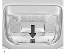
ightharpoolube : Press this button on the overhead console to make the front and rear turn signal lamps flash on and off. This warns others that you are having trouble. Press again to turn the flashers off.
