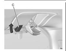
4. While holding the rear glass in place, press the glass-catch release button (C) and pull the top of the rear glass toward you using the grab handles (B) located at the top of the rear glass.
