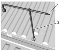
Assembly the wheel wrench (1) and wheel wrench adapter (2), and fit over the hexagon bolt as shown.
