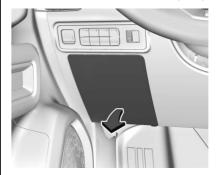
The instrument panel fuse block is on the driver side of the instrument panel, between the steering wheel and the door. To access the fuses, remove the panel, starting at the bottom. Once clips are disengaged, the tabs along the top of the door can be disengaged from the instrument panel to remove the door.
