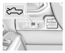
To open the hood, press on the instrument panel to the left of the steering wheel.
