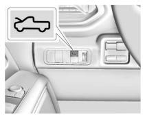
To open the hood, press con the instrument panel to the left of the steering wheel.
