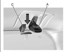
Squeeze and pull down the glass latch levers (A), located near the upper corners of the rear glass, to unlatch. Once unlatched, the glass-catch release button (C) will catch the rear glass and prevent it from falling forward.
