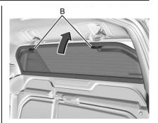
With the rear glass tilted at an angle, place the bottom edge in the lower channel of the window frame.
