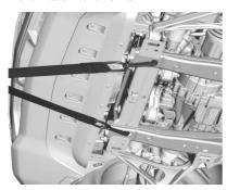
The vehicle is equipped with specific attachment points to be used to pull the vehicle onto a flatbed car carrier from a flat road surface. Do not use these attachment points to pull the vehicle from snow, mud, sand, or ditch.
