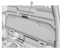
Push the glass against the glass stow retainer (D), located on the interior side of the door. Push until the glass handle slides down to lock the glass in place.
