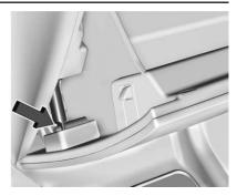
2. Push the dampener arm to the left until it releases the glove box.
