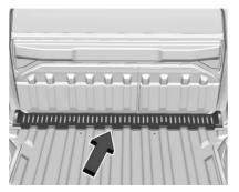
The removable midgate drain grate is located near the base of the midgate.
