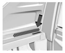
The top drain grates are located near the rear window on both sides of the vehicle. Clean the grates and drains if there is a blockage.
