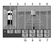
Touch the camera view icons along the bottom of the infotainment display to access each view:
