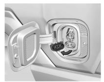
5. Plug in the DC charge cord into the vehicle charge port. Make sure that the DC vehicle plug is fully connected to the DC charge port. If it is not properly connected, the vehicle may not be charged. Check the Driver Information Center (DIC) to make sure the vehicle plug is connected properly.
