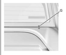
Be sure to align the rear glass side-to-side using the glass alignment arrows (G).
