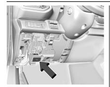
Insert the SD card into the card reader under the instrument panel fuse cover to the left of the steering wheel. See Instrument Panel Fuse Block (Left) ⇒ 340 or Instrument Panel Fuse Block (Right) ⇒ 342. Disable the system from the playback screen before removing the SD card from the reader. Do not remove the card while recording is enabled. This could corrupt the video file and/or the SD card.
