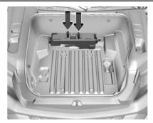
Loosen and remove the two retainers by turning counterclockwise. Remove the jack and tools. Place the jack near the tire being changed.
