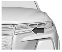
The headlight CSI bar is located on the headlamps. As charging occurs, the blue light bars on the headlamps fill towards the center of the vehicle.
