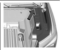
3. Turn the three bolts three quarter turn and remove the right side access cover.
