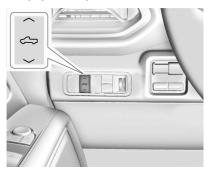
Press either "Up" or "Down" Ride Height button to open the Ride Height menu. Select the desired ride height from the following
