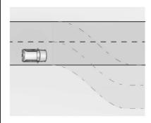
Super Cruise may occasionally provide an alert and/or steering that is considered unnecessary. It could respond to lane markings in different lanes, signs, guardrails, and other stationary objects when entering or exiting a curve. This is normal operation. The vehicle does not need service.
