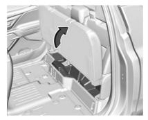
Lift up on the seat bench to access. Push the seat bench down to close.
