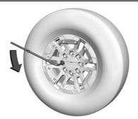
Turn the wheel wrench counterclockwise to loosen all the wheel nuts, but do not remove them yet.
