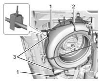
7. Lift the spare tire cage (2) slightly and manually disengage both hook ends (3). For easier disengagement of the hook ends, insert the chisel end of the wheel wrench into one of the tubes (1) and apply upward pressure while disengaging the hook. Do this to both sides.
