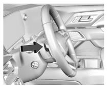
If equipped, Regen on Demand allows increased deceleration by pressing and holding the steering wheel paddle. It works in D (Drive) and L (Low). The accelerator pedal can be used to manage deceleration while using Regen on Demand. See One-Pedal Driving \$\triangle 203.
