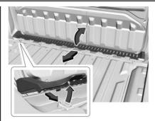
After hauling dirt, wood chips, pebbles etc. the midgate drain should be flushed with water. First remove the drain grate:
