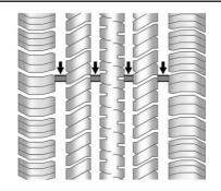
Treadwear indicators are one way to tell when it is time for new tires. Treadwear indicators appear when the tires have only 1.6 mm (1/16 in) or less of tread remaining. See *Tire Inspection* ⇔ 355 and *Tire Rotation* ⇔ 356.
