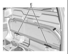
Load the rear glass into the storage pocket in the midgate, guiding the lower edge of the rear glass behind the two rear glass retaining tabs (E).
