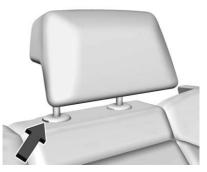
The vehicle's rear seat has adjustable headrest in the center seating position. Pull the headrest up to raise it. Try to move the headrest to make sure that it is locked in place.
