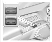
The power windows work when the vehicle is on or when Retained Accessory Power (RAP) is active. See *Power Modes*
