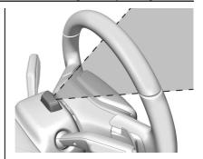
Sunglasses, hats, or other types of clothing that change the shape of the head may interfere with camera performance. To improve camera performance, raise or lower the steering wheel, or change the seat position.
