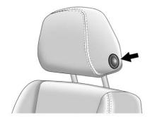
To raise or lower the head restraint, press the button on the side of the head restraint and pull up or push the head restraint down and release the button.
