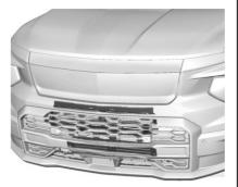
The vehicle may have a shutter system that automatically closes the frontal cooling openings. This system promotes airflow around the vehicle, reducing drag and providing energy savings. Ensure the shutter system is clear of any visible debris, snow, or ice. If the Service Vehicle Soon light activates and remains after clearing the shutter system, see Service Vehicle Soon Light (Propulsion System Failure) \Rightarrow 115.
