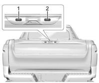
Press Button 2 to open the primary tailgate. Use the top of the tailgate to pull against if additional force is required.
