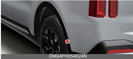
Rear side ultrasonic sensors
