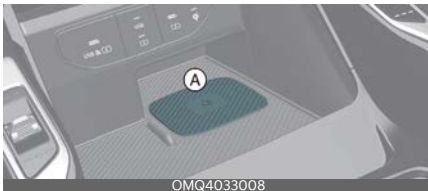
A: Charging pad
