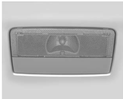
Center Dome Lamp
