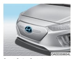
Smart Cruise Control uses a sensor to detect distance to the vehicle ahead.
