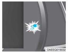
Check if the charging indicator light of the high voltage battery in the instrument cluster is turned ON. Charging is not done when the charging indicator lamp is OFF.
