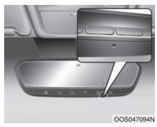
The Compass can be turned ON and OFF, but it returns to ON after the ignition is cycled.
