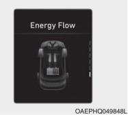
The high-voltage battery is charged up by the regenerative brake system.
