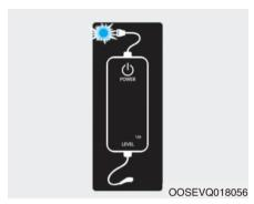
2. Check if the power lamp (green) illuminates on the control box.
