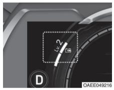
While using the regenerative brakes, you may select the regenerative braking rate from 0 to 3 by pulling the paddle shifter.
