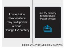
[A]: Displays when turning off vehicle. [B]: Displays when turning on vehicle.
