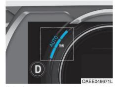
If the front radar recognizes the vehicle in front, 'AUTO' is displayed in blue. The regenerative braking level is automatically controlled depending on the driving condition of the vehicle in front and the level is indicated with arrows.
