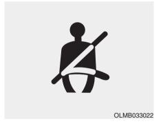
As a reminder to the driver, the seat belt warning light will illuminate and warning chime will sound for approximately 6 seconds each time you turn the POWER button ON if the seat belt is unfastened. If you continue not to fasten the seat belt and you drive over 6 mph (9 km/h), the warning light will stay illuminated.
