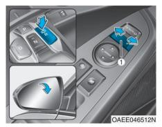
When you shift the vehicle to R (Reverse) position, the side view mirror(s) will rotate downwards to aid with driving in reverse. The position of the side view mirror switch (1) determines whether or not the mirrors will move:
