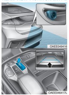
Rear View Monitor system is a supplemental system that shows the area behind the vehicle on the infotainment system screen to assist you when parking or driving.
