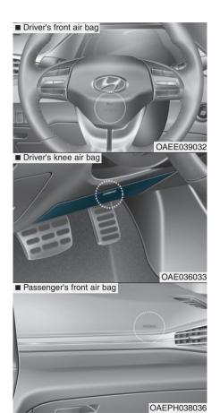
The purpose of the SRS is to provide the vehicle's driver and front passengers with additional protection than that offered by the seat belt system alone. The advanced SRS offers the ability to control the air bag inflation within two levels. A first stage level is provided for moderate-severity impacts. A second stage level is provided for more severe impacts.
