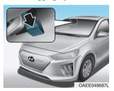
Auto defogging system reduces the possibility of fogging up the inside of the windshield by automatically sensing the moisture of inside the windshield.
