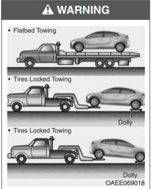
If towing is required, lift all four wheels off the ground and tow the vehicle. If you must tow the vehicle using only two wheels, lift the front wheels off the ground and tow the vehicle
