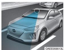
Lane Keeping Assist system helps detect lane markers on the road with a front view camera at the front windshield, and assists the driver's steering to help keep the vehicle between lanes
