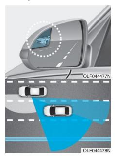
The Blind Spot Mirror (BSM) is a supplemental mirror that reduces the driver's blind spot by showing the rear side area of the vehicle. The blind spot mirror is equipped on the left-hand side view mirror.
