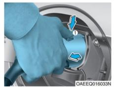
2. Hold the charging connector handle and pull it while pressing the release button (1).
