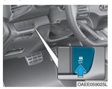
The Electronic Stability Control (ESC) system helps to stabilize the vehicle during cornering maneuvers.
