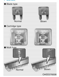
A vehicle's electrical system is protected from electrical overload damage by fuses.
