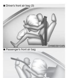
After complete inflation, the air bag immediately starts deflating, enabling the driver to maintain forward visibility and the ability to steer or operate other controls.
