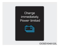
When the high voltage battery level reaches below 6%, this warning message is displayed.
