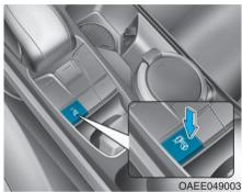
When the POWER button is in the ON position or when the vehicle is in the ready ( ) mode, press the heated steering wheel button to warm the steering wheel. The indicator on the button will illuminate.
