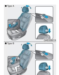
To reinstall the head restraint:
