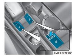
While the vehicle is in the ready ( ) mode, push either of the switches to warm the driver's seat or front passenger's seat.
