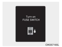
This warning message is displayed if the fuse switch under the steering wheel is OFF.
