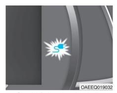
11. Check if the charging indicator light of the high voltage battery in the instrument cluster is turned ON. Charging is not done when the charging indicator lamp is OFF.
