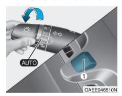
Adaptive front lighting system uses the steering angle and vehicle speed, to keep your field of vision wide by swiveling and leveling the headlamp. Change the switch to the AUTO position when the vehicle is in the ready ( ) mode. The adaptive front lighting system will operate when the headlamp is ON. To turn off the AFL system, change the switch to other positions. After turning the AFL system off, headlamp swiveling no longer occurs, but leveling operates continuously.
