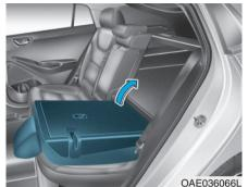
7. To use the rear seat, lift and unfold the seatback to the upright position. Push the seatback firmly until it clicks into place. Make sure the seatback is locked in place.
