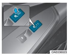
While the vehicle is in the ready ( ) mode, push either of the switches to warm the rear seat.
