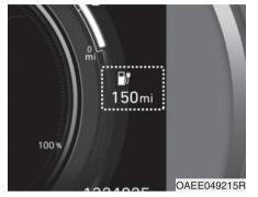
The distance to empty is the estimated distance the vehicle can be driven with remaining level of the high voltage battery.
