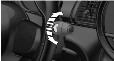
Turn the thumbwheel on the wiper lever.
