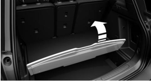
2. Grasp the cargo floor panel at the rear and fold it upward.
