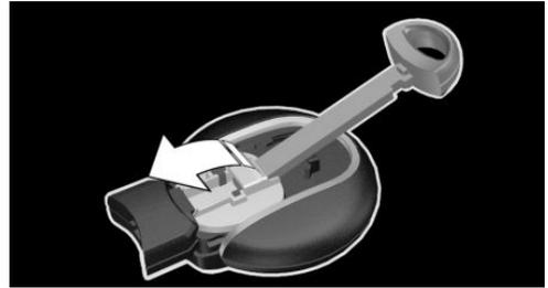
4. Push battery in arrow direction using a pointed object and lift it out.
