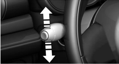
With radio-ready state switched off, press the lever either up or down past the resistance point for approx. 2 seconds.
