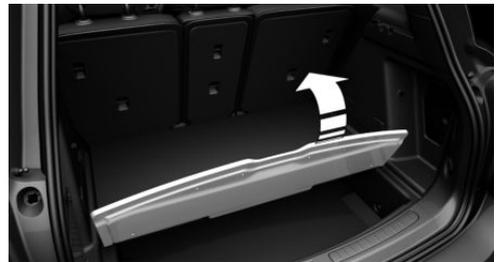
2. Place the MINI Picnic Bench on the front part of the cargo floor panel and at-
