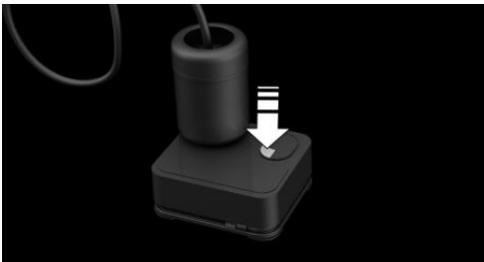
Let the compressor run for max. 10 minutes to fill the tire with sealing compound and achieve a tire inflation pressure of approx. 2.5 bar.
