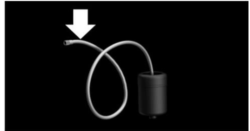
3. Slide the sealant bottle into the mount on the compressor housing, ensuring that it engages audibly.
