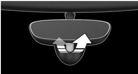
To reduce the blinding glare of the interior mirror, flip the lever forward.
