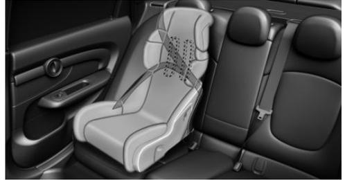
The rear seat belts and the front passenger seat belt can be permanently locked to fasten child restraint systems.
