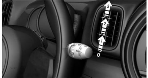
Press the lever up until the desired position is reached.
