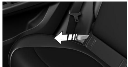
Pull the loop and apply your weight to the backrest or lift it off, as necessary.
