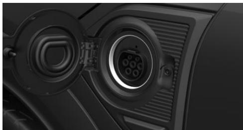
An indicator light is located on the charging socket.
