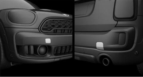
Threaded holes for the tow fitting are located in the front and rear of the vehicle on the right side with respect to the driving direction.
