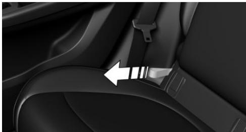
Pull the loop. The rear seat backrest folds forward.
