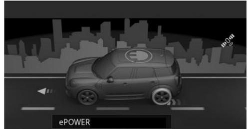
Example: residential area or area with low speed limits. ePOWER electric driving is prepared before the residential area. When the residential area is reached, electric driving is preferred.
