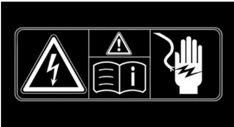
The symbols on parts of the vehicle indicate that incorrect use of high-voltage technology or of orange-colored high-voltage com-
