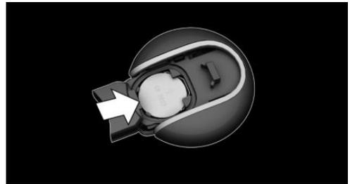
5. Insert a type CR 2032 3V battery with the positive side facing up.
