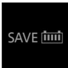
The current charge state of the high-voltage battery can be maintained or increased with SAVE BATTERY. The electric range can be conserved in this way for a later point in the trip, for instance.
