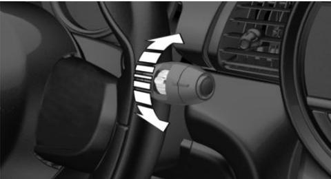
Turn the thumbwheel on the wiper lever.
