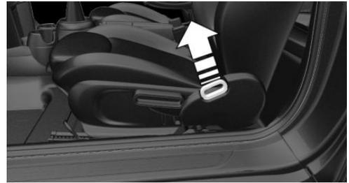
Pull the lever, and apply your weight to the backrest or lift it off, as necessary.
