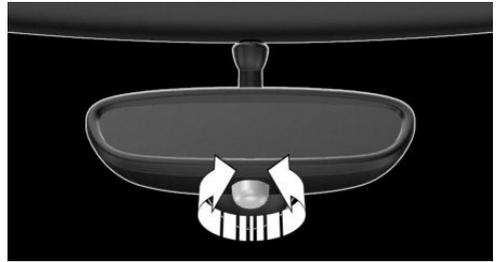
Turn the button to reduce the blinding glare by the interior mirror.
