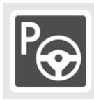
The parking operation is active. The system takes over the steering.
