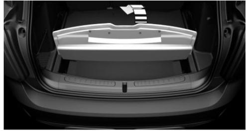
2. Grasp the MINI Picnic Bench in the middle and pull it back and up against the resistance of the magnets.
