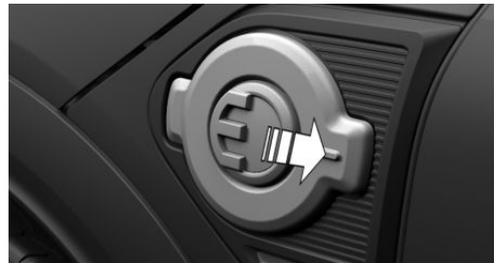
2. Remove the cover of the charging cable connector, if needed.
