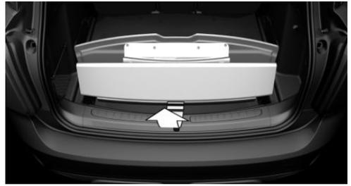
3. Fold the rear part of the cargo area floor downward and place the MINI Picnic Bench over the loading lip of the cargo area. Place a protective cloth over the bumper.
