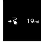
In MAX eDRIVE mode, the electric range can be displayed via the trip computer in the instrument cluster.
