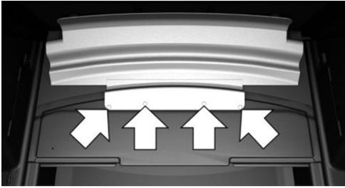
3. Fold down the MINI Picnic Bench toward the rear. The MINI Picnic Bench is fastened with magnets.
