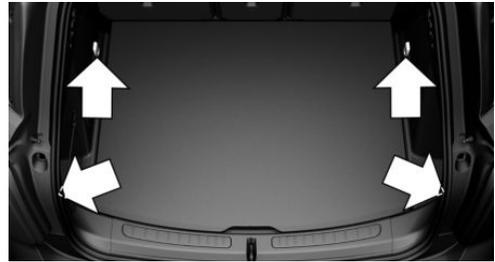
With storage compartment package: to secure the cargo there are four lashing eyes in the cargo area.
