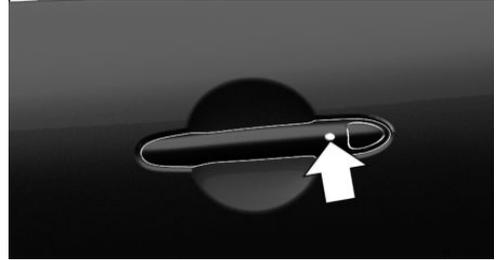
Press and hold down the button on the external door handle of the driver's or front passenger door.
