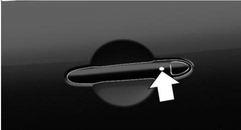
Press the button on the external door handle of the driver's or front passenger door.
