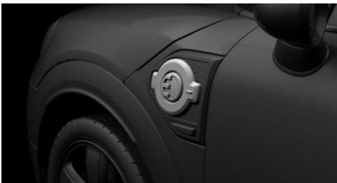
The charging socket cover is located on the left side of the vehicle.
