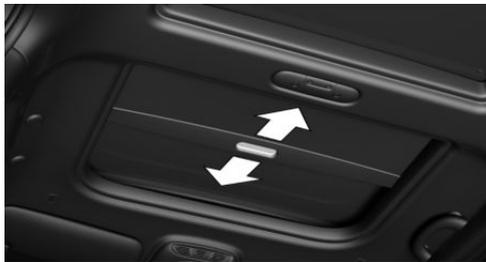
Use the handle to slide the sun protection into the desired position.
