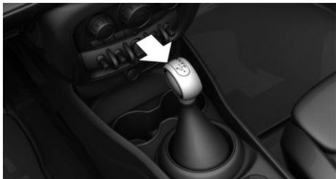
2. Move the selector lever into the desired position.
