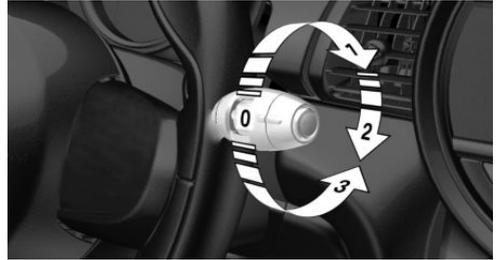
Turn the outer switch upward.
