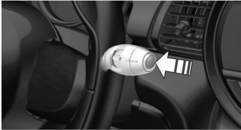
Press the button on the wiper lever.
