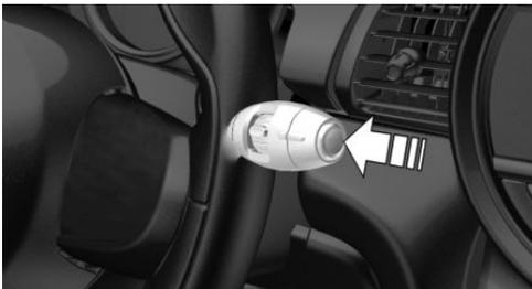
Press the button on the wiper lever.
