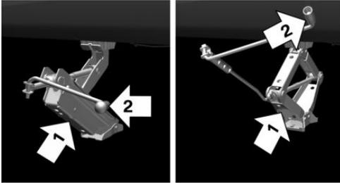
2. Insert the jack into the rectangular recess of the jacking point closest to the wheel to be changed.
