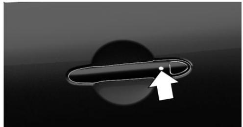
Press the button on the external door handle of the driver's or front passenger door.
