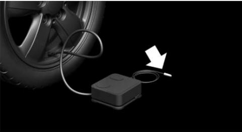
5. With the ignition turned on or the engine running, turn on the compressor and let it run for a maximum of 10 minutes.
