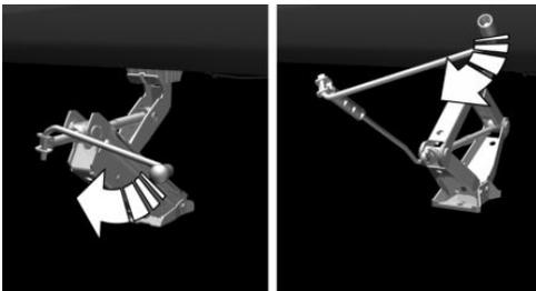
4. Take your hand away from the jack as soon as the jack is under load and continue turning the jack crank handle or lever with one hand.
