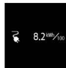
The current electric energy consumption or generation can be monitored.
