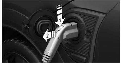
3. Detach the charging cable from the charging socket, arrow 2.
