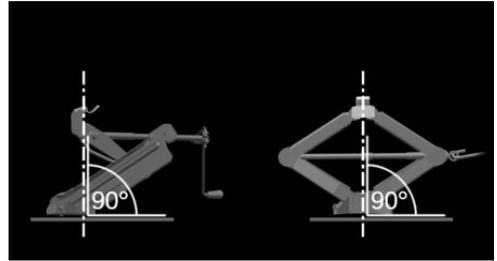
6. Make sure that the car jack foot stands vertically and perpendicularly beneath the jacking point after extending the vehicle jack.
