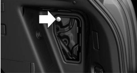
3. To open the fuel filler flap, press on the rear edge. The fuel filler flap opens.
