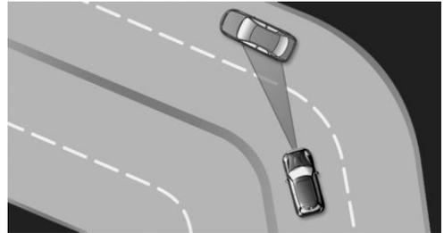
When you approach a curve the system may briefly report vehicles in the next lane due to the bend of the curve. If the system decelerates you may compensate it by briefly accelerating. After releasing the accelerator pedal the system is reactivated and controls speed independently.
