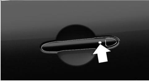
Press the button on the door handle of the driver's or front passenger door.
