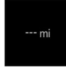
The display indicates that the high-voltage battery is almost fully discharged or the electric drive is currently not available.
