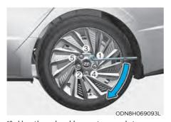
13. Use the wheel lug nut wrench to tighten the lug nuts in the order shown. Double-check each lug nut until they are tight. After changing tires, have an authorized HYUNDAI dealer tighten the lug nuts to their proper torque as soon as possible. The wheel lug nut should be tightened to 79-94 lbf-ft (11-13 kgf-m).
