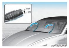
Within 20 seconds of turning off the engine, lift up and hold the wiper lever to the MIST position for about 2 seconds until the wipers move to the top wipe position.
