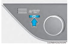
If you press the DRIVER ONLY button (\$\mathbb{G}\text{only}\text{only}\) and the indicator light illuminates, air mostly blows in the direction of the driver's seat.
