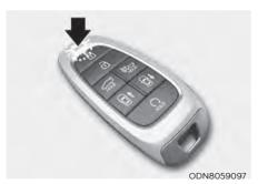
\* When the distance between the smart key and vehicle is over 13 ft. (4 m), the smart key LED may not display normally. You should use it within the operable range.
