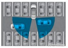
Rear Cross-Traffic Collision-Avoidance Assist monitors approaching cross traffic from the left and right side of the vehicle when your vehicle is approaching.
