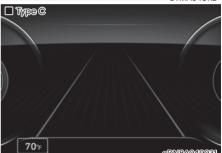
This gauge indicates the current outside air temperature by 1°F (1°C).
