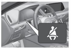
As a reminder to the driver, the seat belt warning light will illuminate for approximately 6 seconds each time you place the ignition switch to the ON position regardless of belt fastening. However, if the seat belt is Unfastened, a warning chime will sound for approximately 6 seconds.
