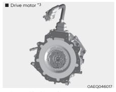
\*3: Located in the engine compartment
