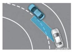
Blind-Spot Collision Avoidance Assist may not operate properly when driving on a curved road. In certain instances, Blind-Spot Collision Avoidance Assist may recognize a vehicle in the same lane.
