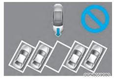
Remote Smart Parking Assist is not a supplemental for diagonal parking. Even if the vehicle is able to enter the space, do not operate the system.
