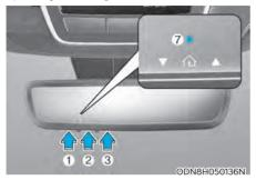
Press and release the HomeLink button (1), (2) or (3), you would like to program. The HomeLink indicator light (7) will flash orange slowly (if not, perform the steps of "Erasing HomeLink Buttons" section, and start over).
