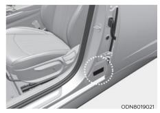
The vehicle certification label attached on the driver's side center pillar gives the Vehicle Identification Number (VIN).
