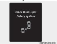
When Safe Exit Warning is not working properly, the 'Check Blind-Spot Safety system' warning message will appear on the cluster, function will turn off automatically function will be limited. Have the vehicle inspected by an authorized HYUNDAI dealer.
