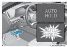
When you stop the vehicle completely by depressing the brake pedal, the Auto Hold maintains the brake pressure to hold the vehicle stationary. The indicator changes from white to green.
