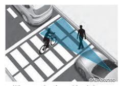
When a pedestrian or bicycle is between you and the vehicle ahead If there is a pedestrian(s) or bicycle(s) in between you and the vehicle in front, Leading Vehicle Departure Alert may not operate properly.
