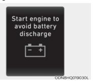
If the engine is not turned on with the Engine Start/Stop button in ACC or ON for a while, the battery can be discharged. Please turn on the engine to prevent 12V battery from discharge.
