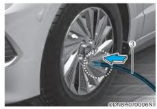
4. Remove the valve cap from the air valve of the damaged tire and connect filling hose (3) of the sealant bottle onto the valve.
