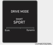
With the standard driving style in the center, the left side of the gauge is 'Econ.' and right side is 'Dynamic' style.
