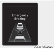
This warning message appears on the LCD display with a warning chime. Additionally, some vehicle function intervention occurs by the engine management system to help decelerate the vehicle.
