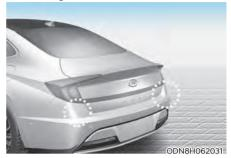
The rear corner radars are sensors located inside the rear bumper to detect the side and rear areas. Always keep the rear bumper clean for proper operation of Safe Exit Warning.
