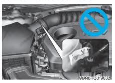
In case of emergency, cut the service interlock connector cable to isolate the high voltage of the battery.
