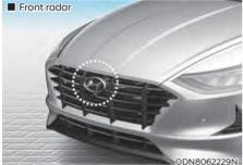
The front radar is a sensor detecting vehicles in front and maintains the distance between them.
