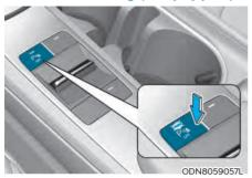
Push the button to turn off Reverse Parking Distance Warning. The indicator light on the button will turn on.
