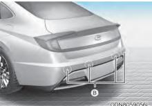
[A]: Front sensor, [B]: Rear sensor
