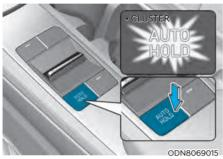
With the driver's door and engine hood closed, depress the brake pedal and then press the [AUTO HOLD] switch. The white AUTO HOLD indicator will come on and the system will be in the standby position.
