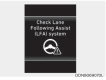
Check LFA (Lane Following Assist) system If there is a problem with the system a message will appear for a few seconds. If the problem continues Lane Following Assist failure indicator will illuminate.
