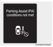
When Remote Smart Parking Assist is not getting ready for activation, the above message will appear when Remote Smart Parking Assist button is pressed.
