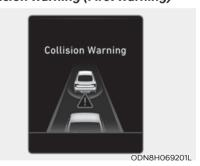
This warning message appears on the LCD display with a warning chime. Additionally, some vehicle function intervention occurs by the engine management system to help decelerate the vehicle.
