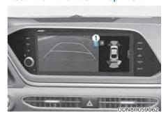
When you touch the icon (1), the top view is displayed on the screen and shows the distance from the vehicle in the back of your vehicle. Touch the icon (1) again, to switch back to the previous screen.
