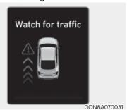
Collision warning when exiting vehicle
