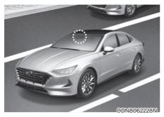
Lane Keeping Assist detect lane markers on the road with a camera at the front windshield, and assists the driver's steering to help keep the vehicle between lanes.
