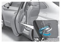
If the electrical power door lock switch is not operating (ex. dead car battery) the only way to lock the door(s) is with the mechanical key from the outside key
