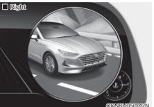
Blind-Spot View Monitor displays the left or right side of the rear blind spot area of your vehicle in the instrument cluster when the left or right turn signal is on. This function helps you when changing lanes.
