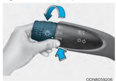
High Beam Assist is a function that automatically adjusts the headlight range (switches between high beam and low beam) according to the brightness of other vehicles and road conditions.
