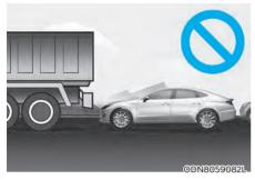
An accident may occur when parking behind a vehicle higher than yours. For example, bus, truck, etc. Do not use the function in that case.
