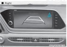
If the risk of collision is detected while Rear Cross-Traffic Collision-Avoidance Assist is generated, brake is controlled. The instrument cluster will inform the driver of the brake control. If the rear view monitor function is in activation, a message will also appear on the infotainment system screen.
