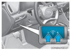
When the vehicle's parking lamps or headlights are on, press the illumination control button to adjust the brightness of the instrument panel illumination.
