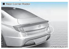
The rear corner radars are the sensors inside the rear bumper for detecting the side and rear areas. Always keep the rear bumper clean for proper operation of Rear Cross-Traffic Collision-Avoidance Assist.
