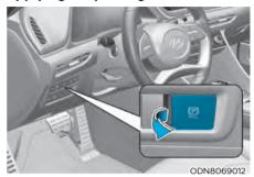
To apply the EPB (Electronic Parking Brake):
