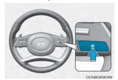
When Smart Cruise Control is ON, you can set and maintain the distance from the vehicle ahead of you without pressing the accelerator or brake pedal. Each time the button is pressed, the Headway changes as follows:
