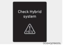
This message is displayed when there is a problem with the hybrid control system. Refrain from driving when the warning message is displayed.
