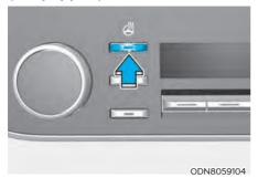
When the ignition switch is in the ON position or when the engine is running, press the heated steering wheel button to warm the steering wheel. The indicator on the button will illuminate.
