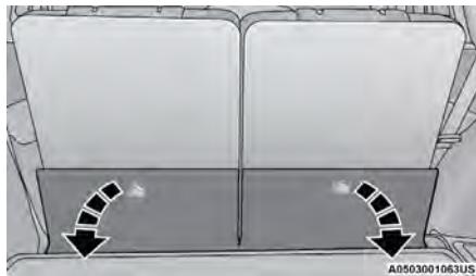
Pulling Down The Carpet Floor Panel To Access Top Tether Strap Anchorage (3rd Row Bench)
