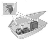
The cargo management system is used to organize storage in the cargo area. There are two convenience hooks that can support up to 5 kg (11 lb).
