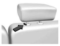
The height of the head restraint can be adjusted. Pull the head restraint up to raise it. Try to move the head restraint to make sure that it is locked in place.
