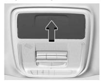
Sunglasses storage is on the overhead console. Press the cover and release to access.
