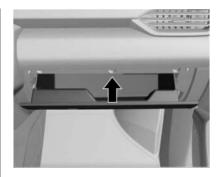
Push the rear center area of the glove box to lower beyond the stops.
