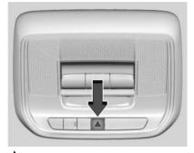
: Press this button on the overhead console to make the front and rear turn signal lights flash on and off. This warns others that you are having trouble. Press again to turn the flashers off.
