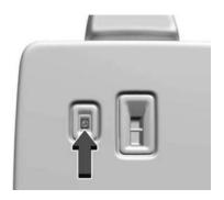
If equipped with power rear seats, the second row seat can also be moved for third row entry/exit by pressing the switch on the second row seat side or on the seatback of the second row seat.
