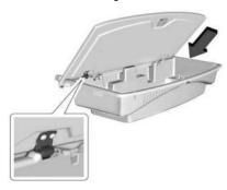
Angle the load floor approximately 70%, align the two hooks on the load floor above the rod, and push the load floor until the hooks engage the cargo bin rod.
