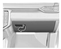
Pull up on the glove box lever to open it.
