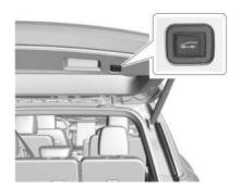
Press on the bottom of the liftgate to close.
