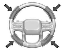
To begin steering manually, hold the steering wheel firmly with both hands using the highlighted regions. The Super Cruise light 🕣 is lit red on the instrument cluster and a message displays in the DIC. In addition, beeps will sound, or the Safety Alert Seat will vibrate. To view Collision and Detection options from the infotainment screen, touch Settings > Vehicle > Collision/Detection Systems. After you begin steering manually, then Super Cruise will disengage.
