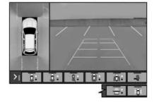
Touch the camera view buttons along the bottom of the infotainment display. Available views will differ depending on vehicle options.
