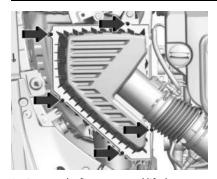
Remove the five screws and lift the cover out of the assembly.
