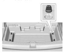
Remove the four wing nuts, then remove the cargo management system. See Cargo Management System \$ 87.
