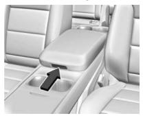
The center console has storage under the armrest. Press the button and lift to open.
