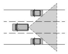
If equipped, this automatic dimming mirror provides a wide angle camera view of the area behind the vehicle.
