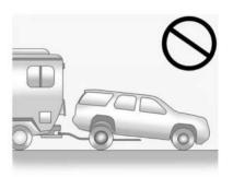
Towing the vehicle from the rear could damage it. Also, repairs would not be covered by the vehicle warranty. Never have the vehicle towed from the rear.
