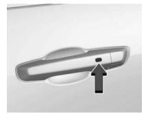
The remote key must be within 1 m (3 ft) of the liftgate or door being opened. Press the button on the door handle to open. See *Remote Key Operation* ♀ 7.
