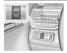
Press the switch to activate the All-Wheel Drive system. The indicator flashes briefly while the system engages and stays lit when the system is active. See *All-Wheel-Drive Light* ▷ 110.
