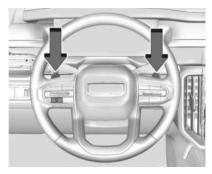
Electronic Range Select, or Manual Mode, allows for the selection of the range of gear positions. Use this mode when driving downhill or towing a trailer to limit the top gear and vehicle speed. The shift position indicator within the Driver Information Center (DIC) will display a number next to the L indicating the highest available gear.
