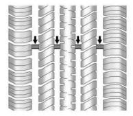
Treadwear indicators are one way to tell when it is time for new tires. Treadwear indicators appear when the tires have only 1.6 mm (1/16 in) or less of tread remaining. See *Tire Inspection* ♀ 301 and *Tire Rotation* ♀ 301.
