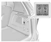
If equipped, the third row seatbacks can also be folded forward and returned to the upright position by pressing and holding the switches on the passenger side of the rear cargo area.
