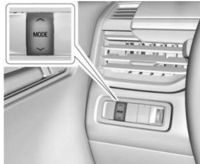
Driver Mode Control Switch
