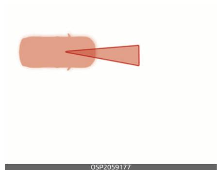
When a vehicle changes lanes in front of you, FCA system may not immediately detect the vehicle, especially if the vehicle changes lanes abruptly. In this case, you must maintain a safe braking distance, and if necessary, depress the brake pedal to reduce your driving speed in order to maintain a safe distance.
