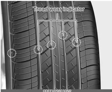
This shows there is less than 1.6 mm (1/16 inch) of tread left on the tire. Replace the tire when this happens.
