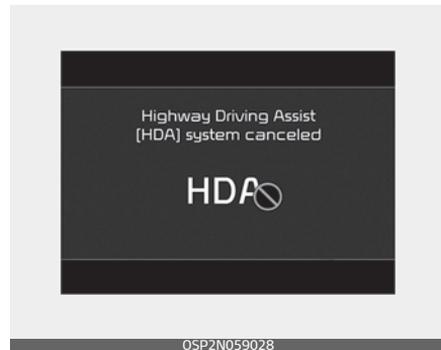
If you keep your hands off the steering wheel even with the hands-off warning on, the steering assist and Smart Cruise Control will be temporarily released automatically.
