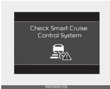
The message will appear when the vehicle to vehicle distance control system is not functioning normally. In this case, take your vehicle to an authorized Kia dealer and have the system checked.
