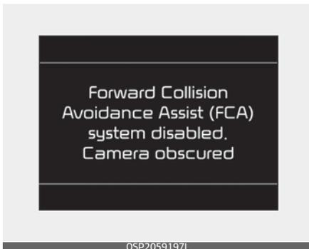
When the camera is blocked with dirt, snow, or debris, FCA system operation may not be able to detect other vehicles.
