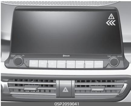
If the vehicle detected by the sensors approaches from the rear left/right side of your vehicle, the warning chime will sound, the warning light on the outside rear view mirror will blink and a message will appear on the LCD display. If the rear view monitor system is in activation, a message will also appear on the infotainment system screen.
