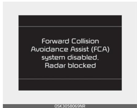
When the sensor cover is blocked with dirt, snow, or debris, FCA system operation may stop temporarily. If this occurs, a warning message will appear on the LCD display.
