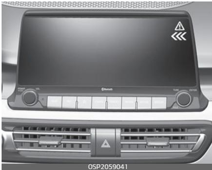
If the risk of collision is detected while RCCW is generated, brake is controlled. The instrument cluster will inform the driver of the brake control. If the rear view monitor system is in activation, a message will also appear on the infotainment system screen.
