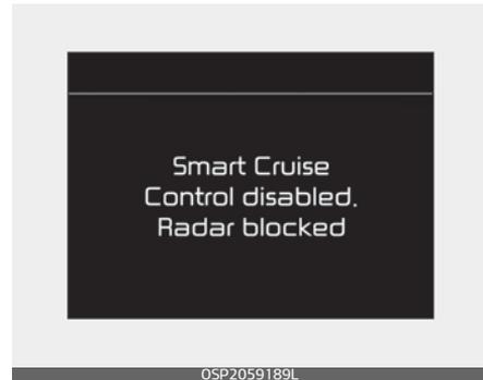
When the sensor lens cover is covered with dirt, snow, or debris, SCC operation may stop temporarily. If this occurs, a warning message will appear on the LCD display. Remove any dirt, snow, or debris and clean the radar sensor lens cover before operating SCC.
