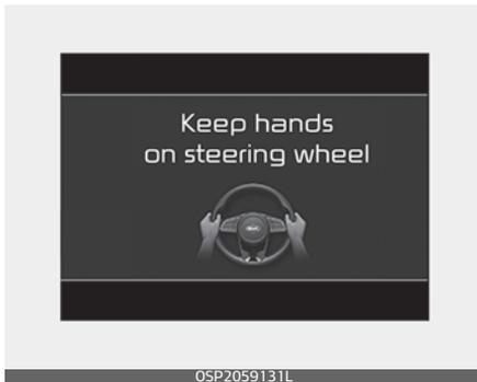
The hands-off warning appears when the system detects that the driver's hands are not on the steering wheel while HDA is in work. (First warning: warning message, Second warning: warning message with warning sound)
