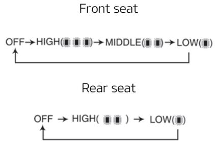
The seat warmer defaults to the OFF position whenever the ignition switch or START/STOP button is turned on.
