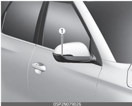
The LED lamps cannot be replaced as a single component because it is an integrated unit. The LED lamps have to be replaced with the unit.
