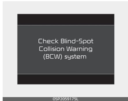
If there is a problem with BCW system, a warning message will appear. The system will turn off automatically. RCCW and RCCA will not operate also if BCW system turns off due to malfunction. You should have the vehicle inspected by an authorized Kia dealer.
