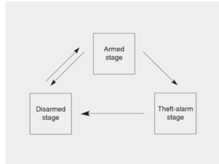
This system is operated in three stages: the first is the "Armed" stage, the second is the "Theft-alarm" stage, and the third is the "Disarmed" stage. If triggered, the system provides an audible alarm with blinking of the hazard warning lights.
