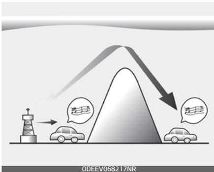
AM broadcasts can be received at greater distances than FM broadcasts. This is because AM radio waves are transmitted at low frequencies. These long distance, low frequency radio waves can follow the curvature of the earth rather than traveling straight. In addition,
