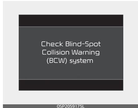
If there is a problem with BCW system, a warning message will appear. The system will turn off automatically. BCA will not operate also if BCW system turns off due to malfunction. You should have the vehicle inspected by an authorized Kia dealer.
