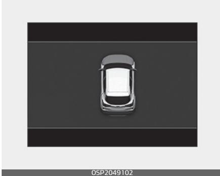
The warning chime will operate when the vehicle is being driven above 3 km/h (2 mph) with the hood open.
