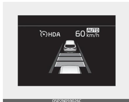
In the automatic speed setting mode, the set speed is automatically adjusted to the changing speed limits of highway sections.
