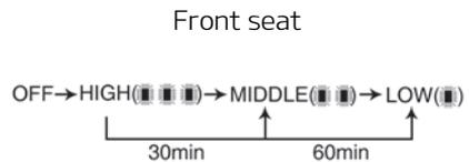
You may manually press the button to increase the seat temperature. However, it soon returns to the automatic mode again. When pressing the switch for more than 1.5 seconds with the seat warmer operating, the seat warmer will turn OFF. The seat warmer defaults to the OFF position whenever the igni-
