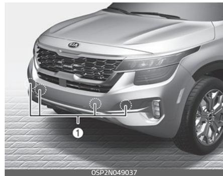
This system is a supplemental system that senses objects within the range and location of the sensors (1), it cannot detect objects in other areas where sensors are not installed.
