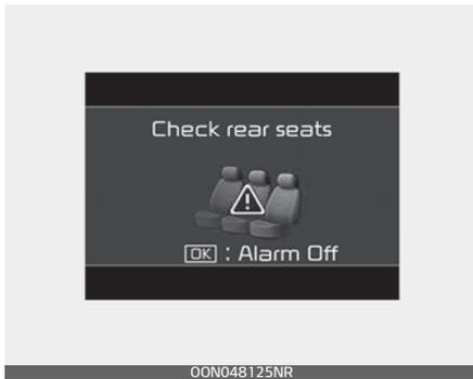
You can activate or deactivate the ROA from the User Settings mode in the cluster LCD display. If your vehicle is equipped with an infotainment system, you can learn how to setup on the website via QR code in the infotainment quick reference guide..
