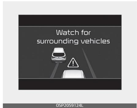
If the vehicle ahead (vehicle speed: less than 30 km/h (20 mph) moves to the next lane, the warning chime will sound and a message will appear. Adjust your vehicle speed for vehicles or objects that can suddenly appear in front of you by depressing the brake pedal according to the road and driving conditions.
