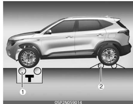
1. Place the front wheels on the roll tester (1) for a speedometer test as shown in the illustration.
