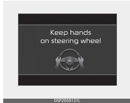
If you keep your hands off the wheel while driving with LFA is in steering assist mode, the hands-off warning will be triggered.
