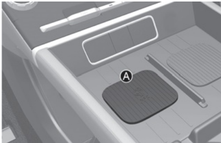
[A] Vehicle authentication pad (wireless charging pad)
