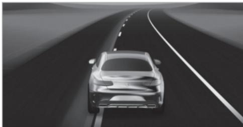
If the front wheel of the vehicle drives over a detected lane marking, this will be highlighted red in the **Assistance** menu on the driver's display.
