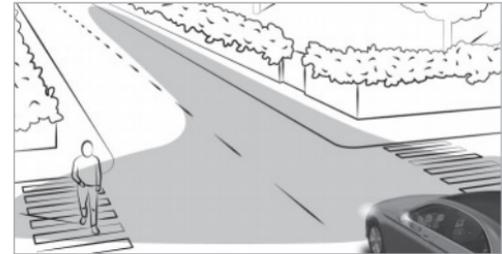
The cornering light improves the illumination of the road over a wide angle in the turning direction, enabling better visibility on tight bends, for example. The cornering light will be activated only when low beam is switched on.
