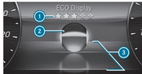
The ECO display shows an evaluation of your driving style on the driver's display depending on the
