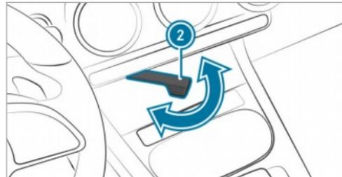
▶ **To secure the mobile phone:** swing lever ② out.
