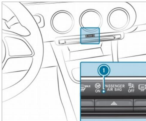
Indicator lamp ❶ will flash when the ATA system is armed.
