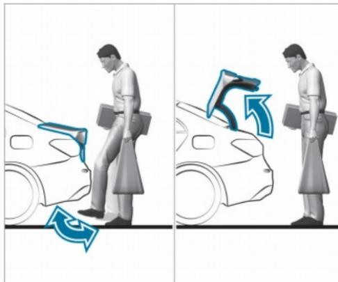
With HANDS-FREE ACCESS you can open the trunk lid by performing a kicking movement under the bumper.
