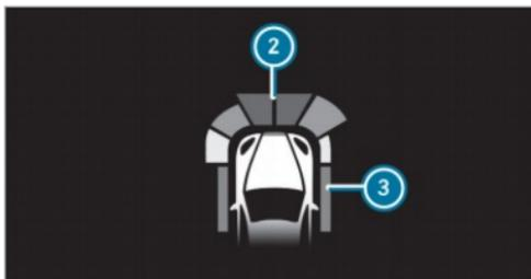
Optionally, obstacles detected by Parking Assist PARKTRONIC from a distance of approximately 3.3 ft (1.0 m) in front ❷ and 2.3 ft (0.7 m) on the side ❸ can also be displayed on the head-up display.
