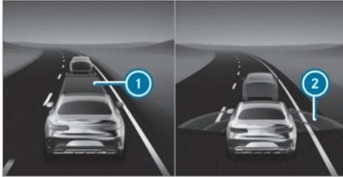
In the **Assistance** menu, an insufficient distance ① to the vehicle in front is displayed in red. If you further reduce the distance, the vehicle in front will also be highlighted in red. When the system detects a risk of collision, red radar waves ② will appear in front of the vehicle.
