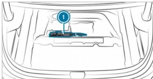
Fuse box ❶ is located in the center underneath
