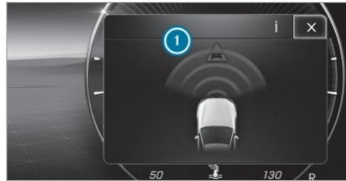
If autonomous braking or situation-dependent brake force boosting has occurred, pop-up ① will appear on the driver's display and then automatically go out after a short time.
