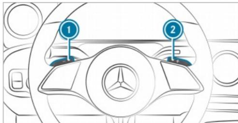
When the automatic transmission is shifted to position **D**, you can manually shift it with the steering wheel paddle shifter. If permitted, the automatic transmission will shift to a higher or lower gear depending on the steering wheel paddle shifter being pulled.
