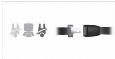
When the vehicle is switched on, the rear seat belt status display informs you for a certain amount of time which rear seat belt is not fastened.
