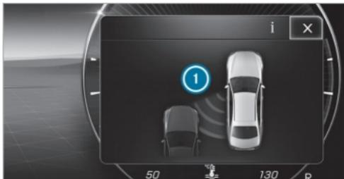
If a course-correcting brake application occurs, the red warning lamp will flash in the outside mirror and a warning tone will sound. In addition, a display ① indicating the danger of a side collision will appear on the driver's display.
