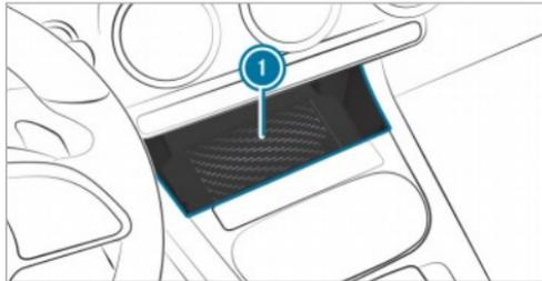
▶ Place the mobile phone as close to the center of the marked surface on mat ① as possible with the display facing upwards. When a message is shown in the multimedia system, the mobile phone is being charged.
