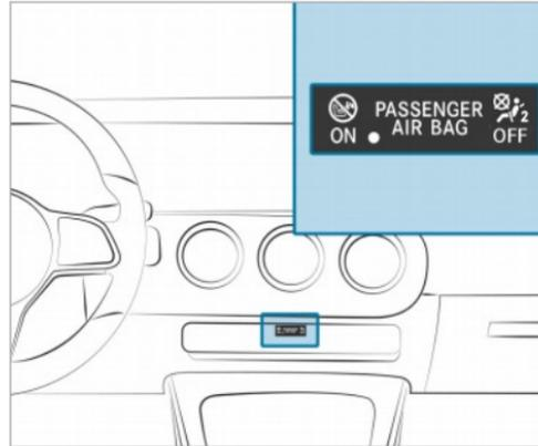
The PASSENGER AIR BAG indicator lamps display the status of the front passenger air bag.
