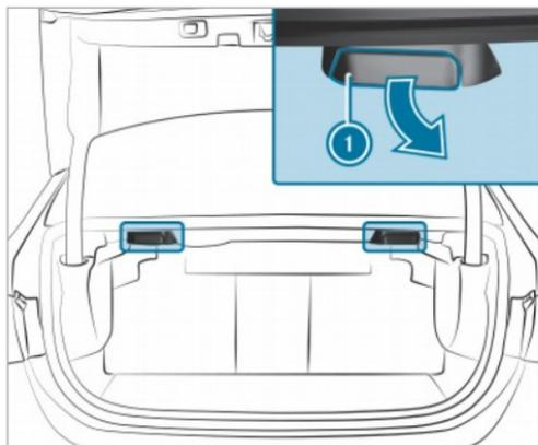
**Vehicles with a memory function:** If necessary, when the seat backrest in the rear passenger compartment is folded forward, the front seat will move forwards slightly to avoid a collision.
