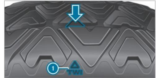
Six marks ① show where the bar indicators (arrow) are integrated into the tire tread. They are visible once a tire tread depth of approximately  $\frac{1}{16}$  in (1.6 mm) has been reached.
