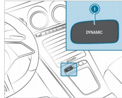
▶ Press DYNAMIC SELECT button **1** as many times as necessary until the selected drive program is displayed in the driver's display.
