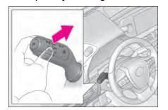
Temporarily switching to the low beams
