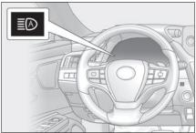
1 Press the Automatic High Beam switch.
