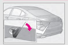
Turn the mechanical key clockwise to open.
