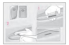
Grip the driver's door handle to unlock the door. Holding the driver's door handle for approximately 2 seconds unlocks all the doors. Grip the passenger's door handle to unlock all the doors.\*
