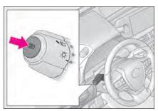
Press the Automatic High Beam switch.
