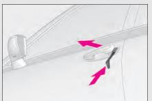
1 Pull the driver's door handle and insert the mechanical key.
