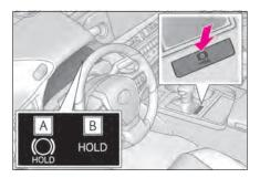
Turns the brake hold system on
