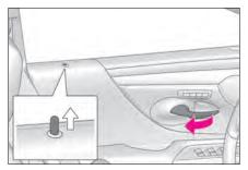
Push down the inside lock button to lock the door.
