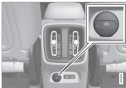
USB ports* (type C) on rear of tunnel console for charging phones, tablets, etc. 7 .
