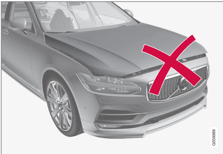
Hood not completely closed.
