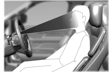
Steering column too high, camera cannot see the face.
