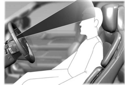
Steering column too high, camera cannot see the face.
